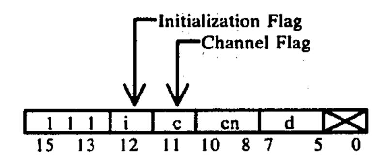
Code (111) transfers the next data word to the window or channel specified by cn (three bits) and the data register specified by the data address field, d (three bits). The word following a transfer code is an initialization data without any code bits.
