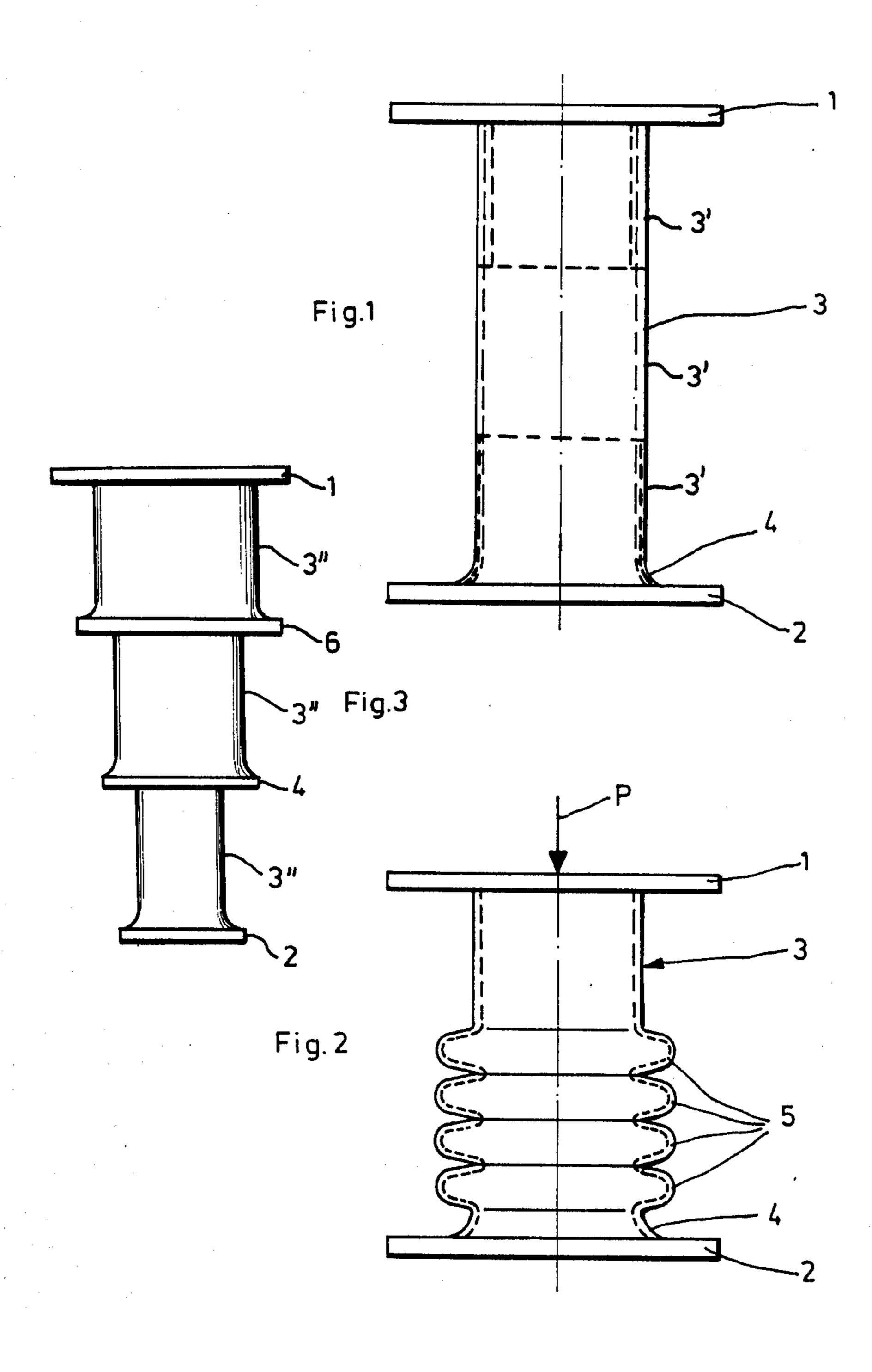
BUMPER ARRANGEMENT FOR VEHICLES WITH AT LEAST ONE DEFORMATION TUBE
