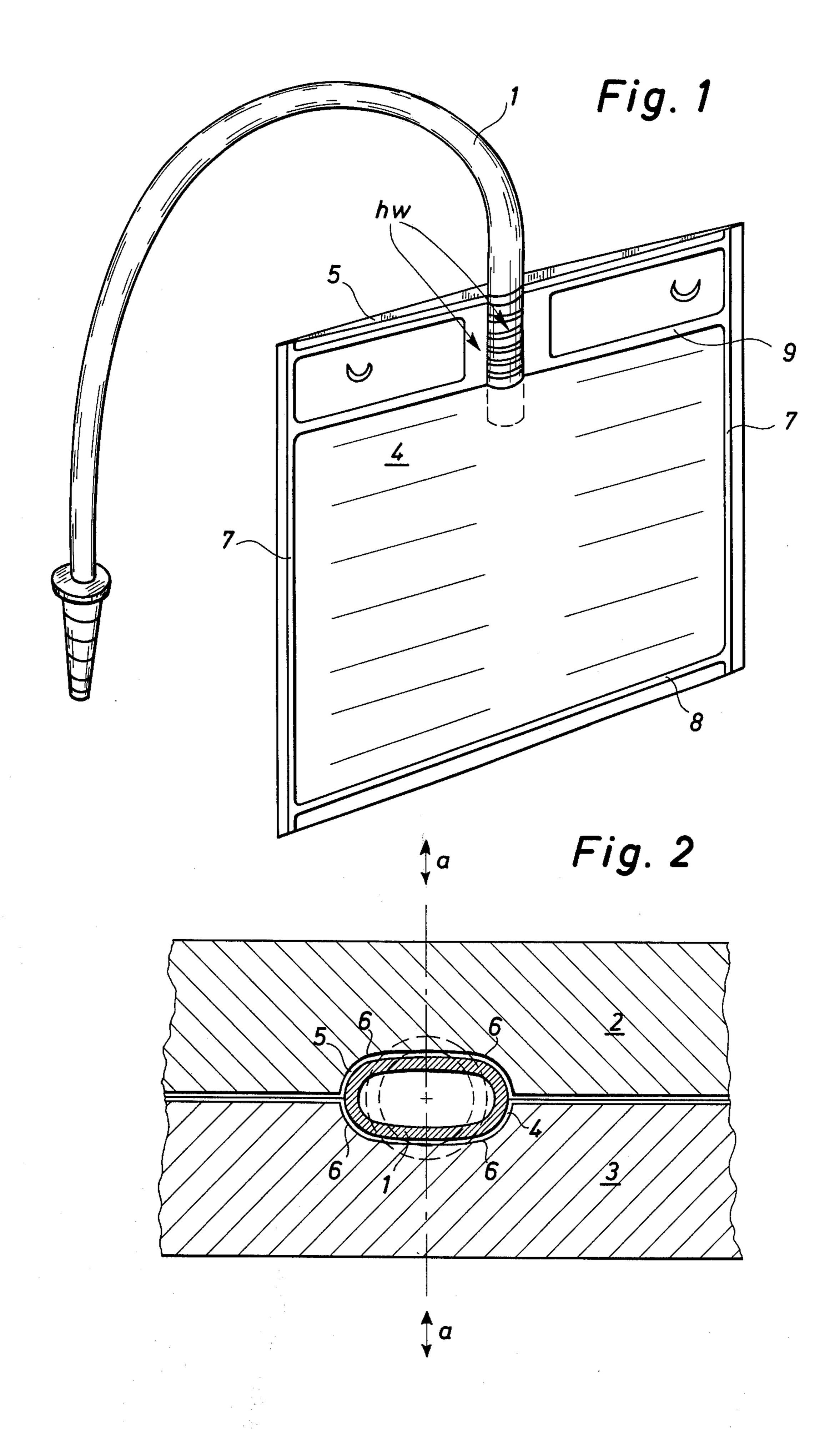
The invention relates to a bag such as a urine bag of polyethylene film consisting of two layers of film 5 welded together along their edges except at an aperture in the upper edge, in which aperture one end of a cylindrical or oval tube of the same material is inserted. The invention also relates to a method of producing the bag.
