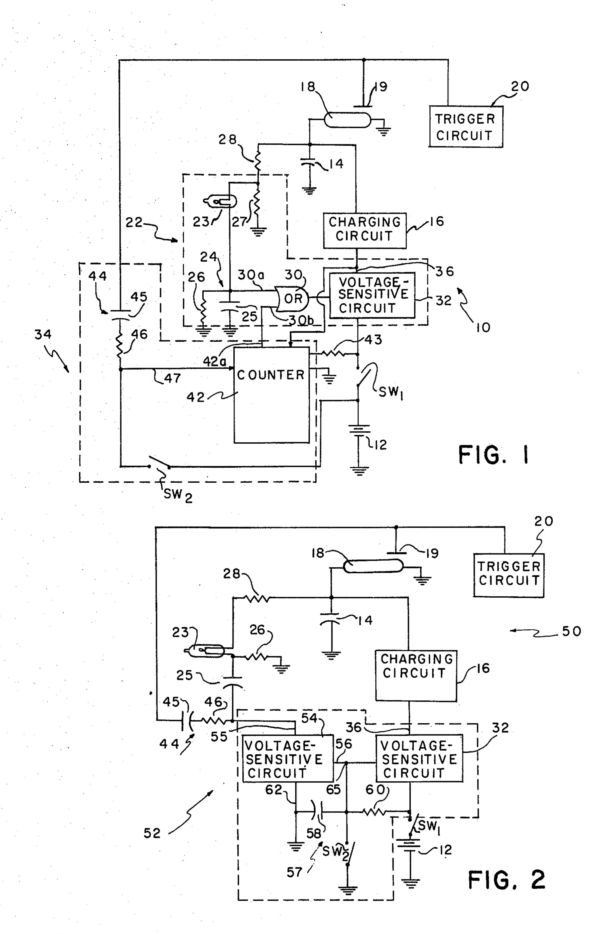
ELECTRONIC FLASH APPARATUS FOR CONSERVING FLASH BATTERY LIFE
