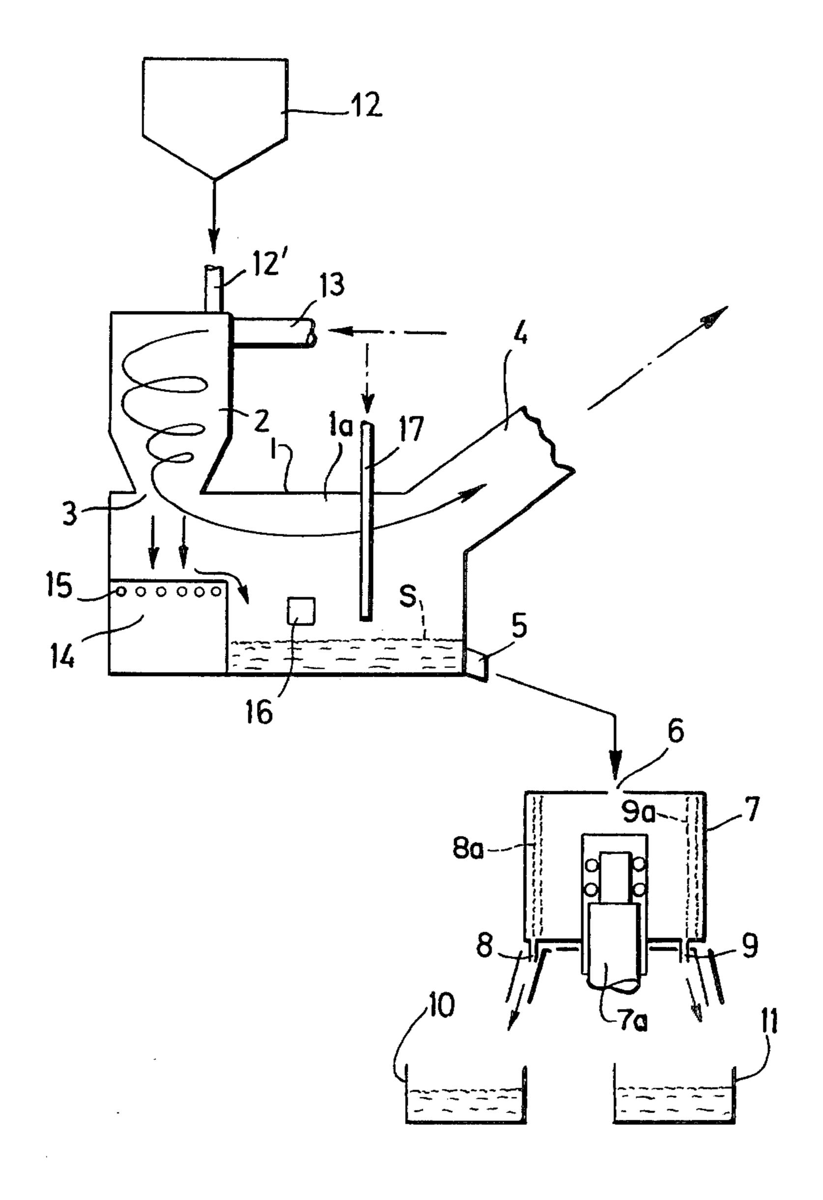
THERMAL METHOD FOR THE RECOVERY OF METALS AND/OR METAL COMBINATIONS WITH THE AID OF A MELTING CYCLONE
