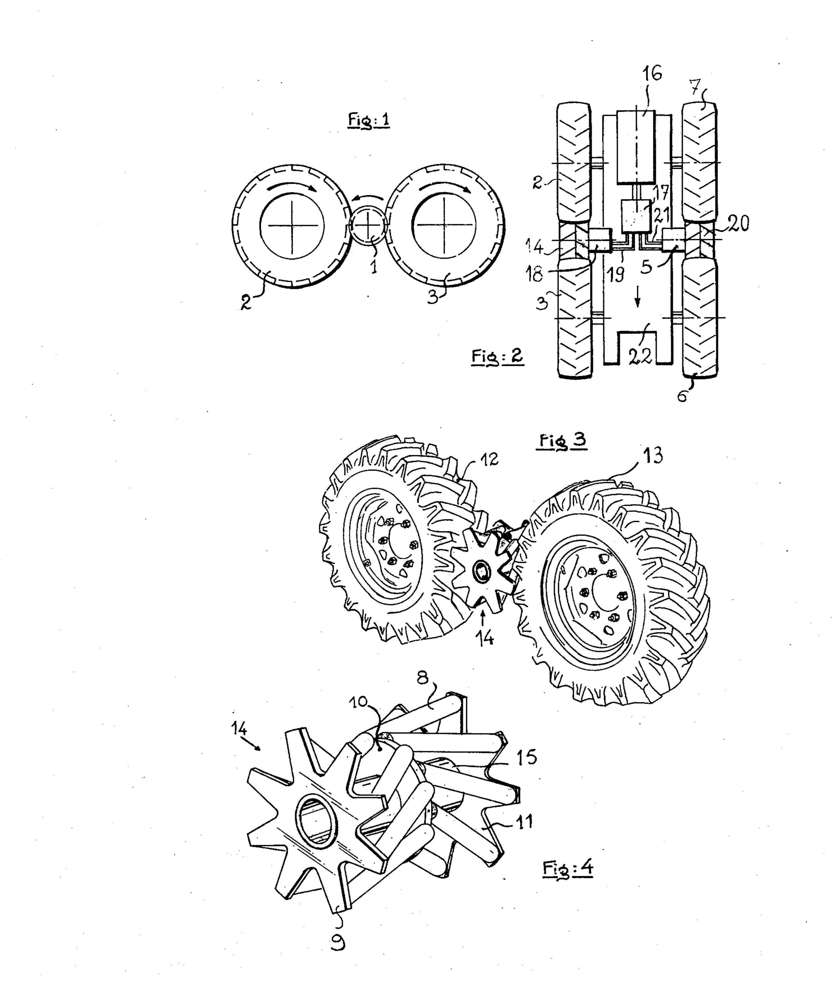
METHOD AND DEVICE FOR DRIVING THE DRIVING WHEELS OF A VEHICLE
