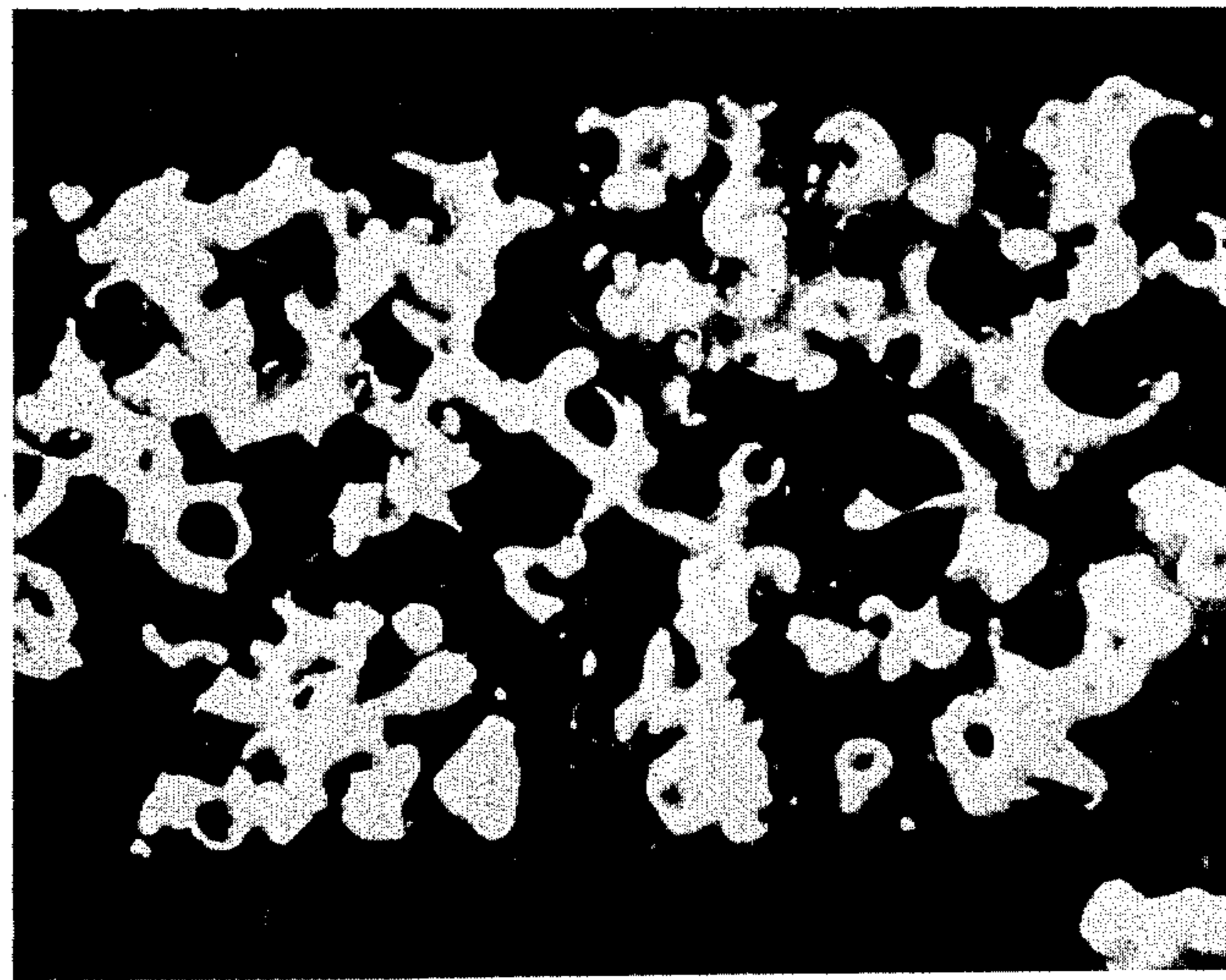
LIQUID PHASE SINTERED POROUS NICKEL SHEET FIG.3
