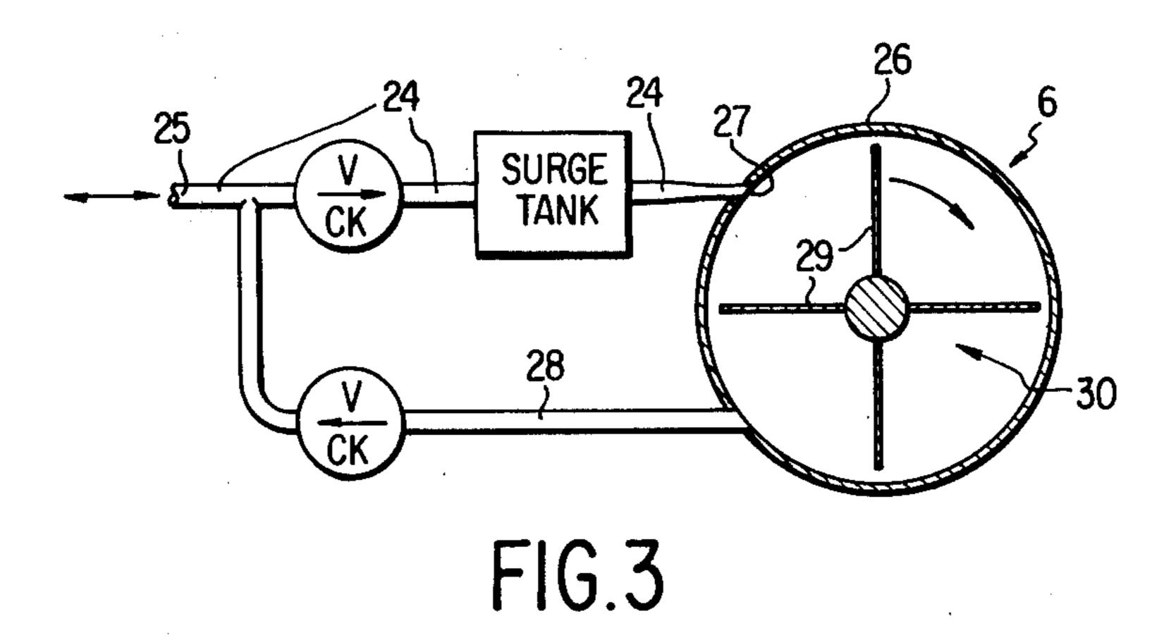
THERMALLY DRIVEN PISTON APPARATUS HAVING AN ANGLED CYLINDER BYPASS DIRECTING FLUID INTO A THERMAL LAG HEATING CHAMBER BEYOND THE BYPASS
