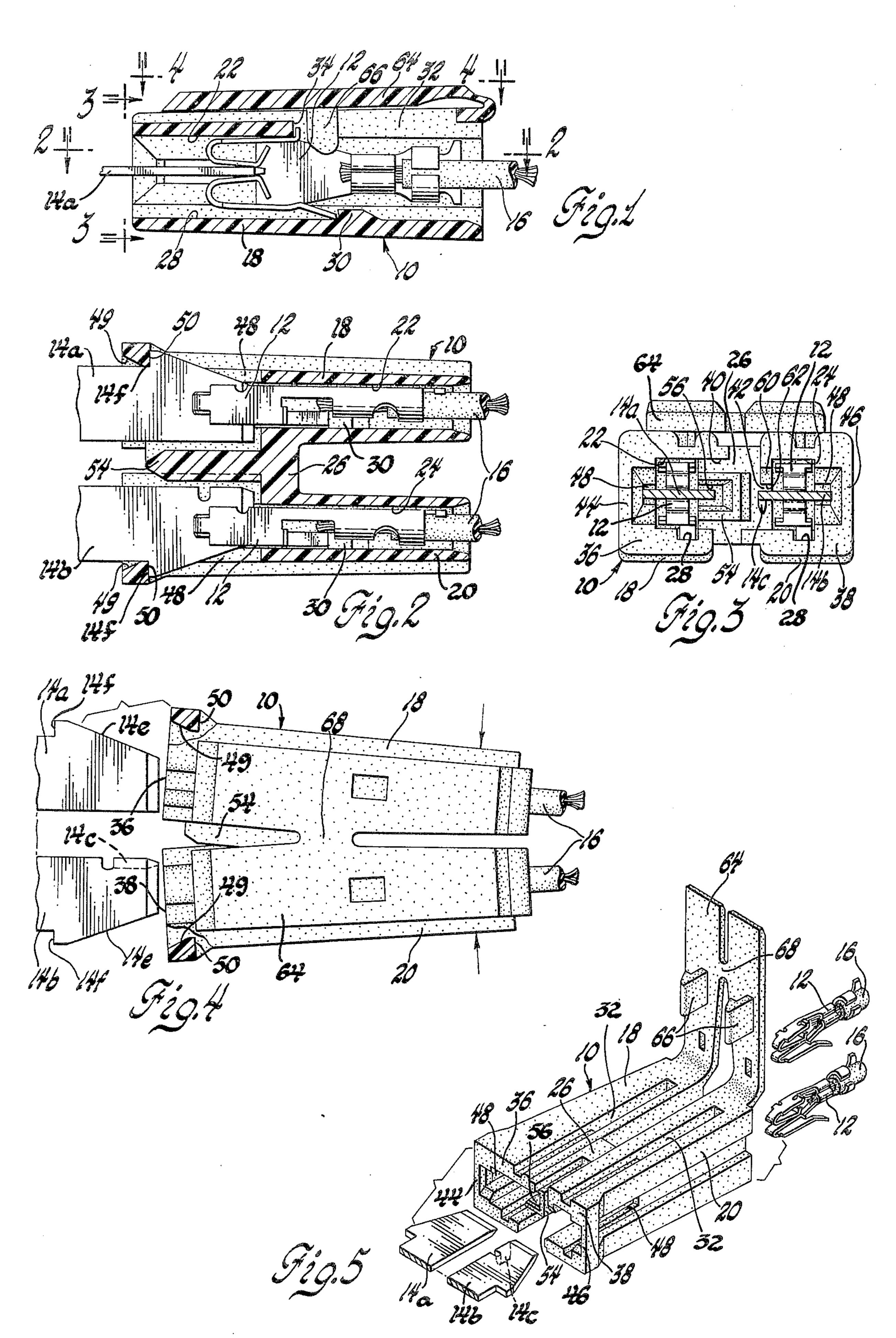
This invention relates generally to electrical connectors and more specifically to electrical connectors having a unitary connector body of molded dielectric ma- 5 terial provided with means for locking the connector body in a coupled position where terminals housed in the connector body are mated with terminals of another electrical device.
