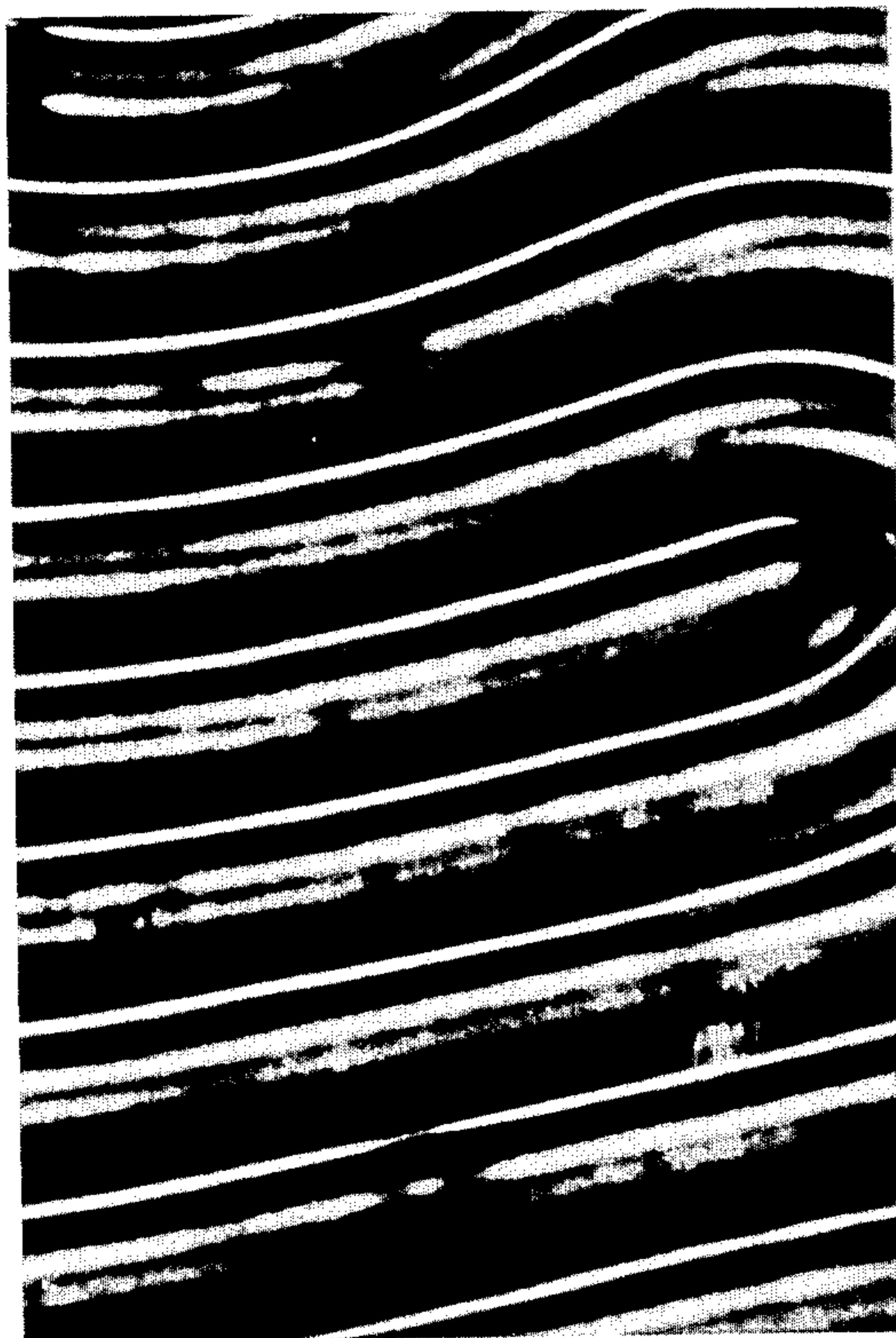
Homeotropically aligned cholesteric phase consisting of 0.7% of cholesteryl-2-methylvalerate in MBBA. Magnification 150x. The pitch of this sample is \approx 105\mu .
