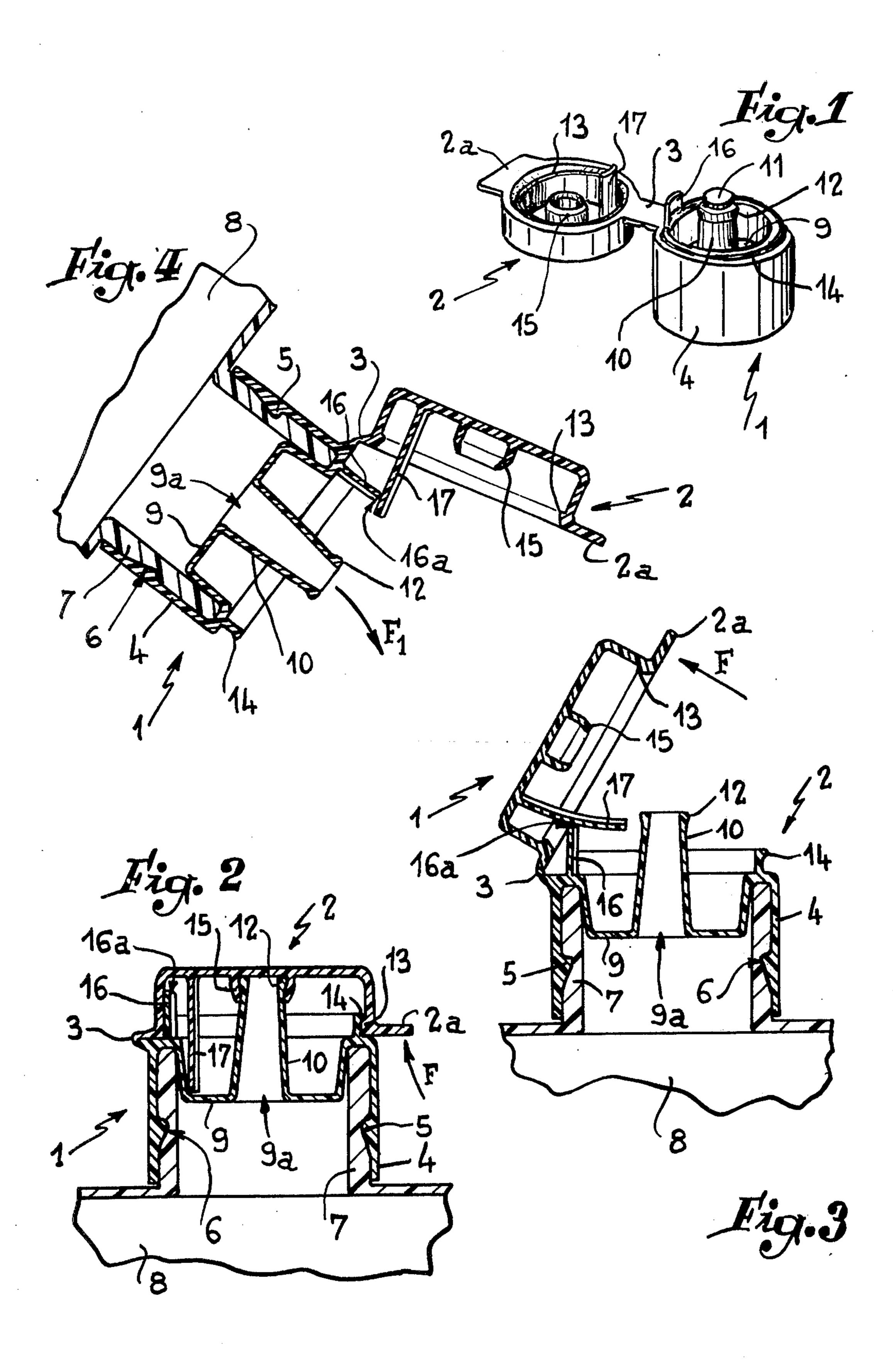
The present invention relates to pourer stoppers more especially intended for use with a container holding a liquid poured by means of a spout having a very small aperture so that the said liquid flows in the form of a jet. Pourer stoppers of this kind are used particularly on containers for liquids such as cleaning materials and syrups.
