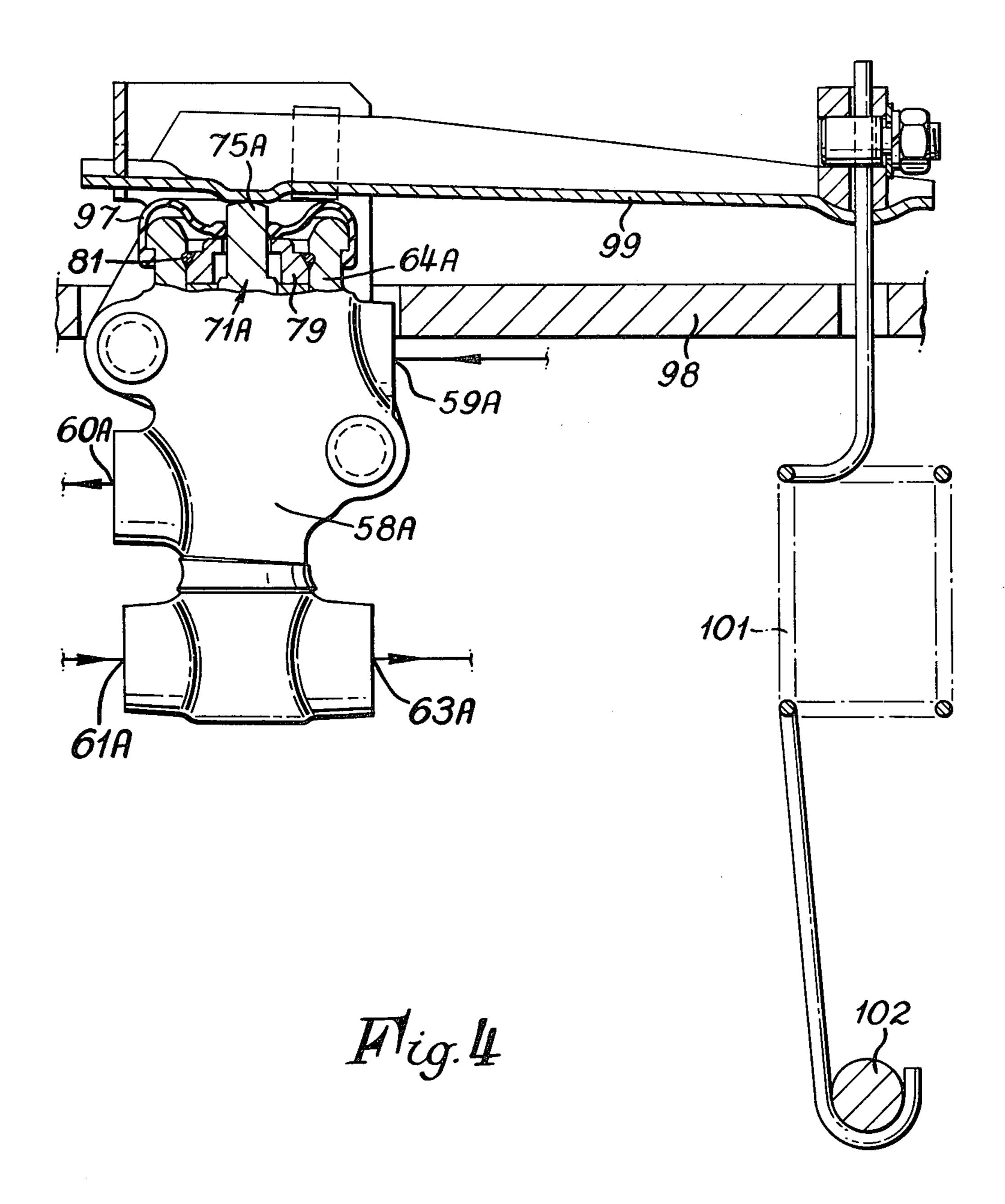
VALVE DEVICES FOR USE IN LIQUID PRESSURE BRAKING SYSTEMS OF VEHICLES
