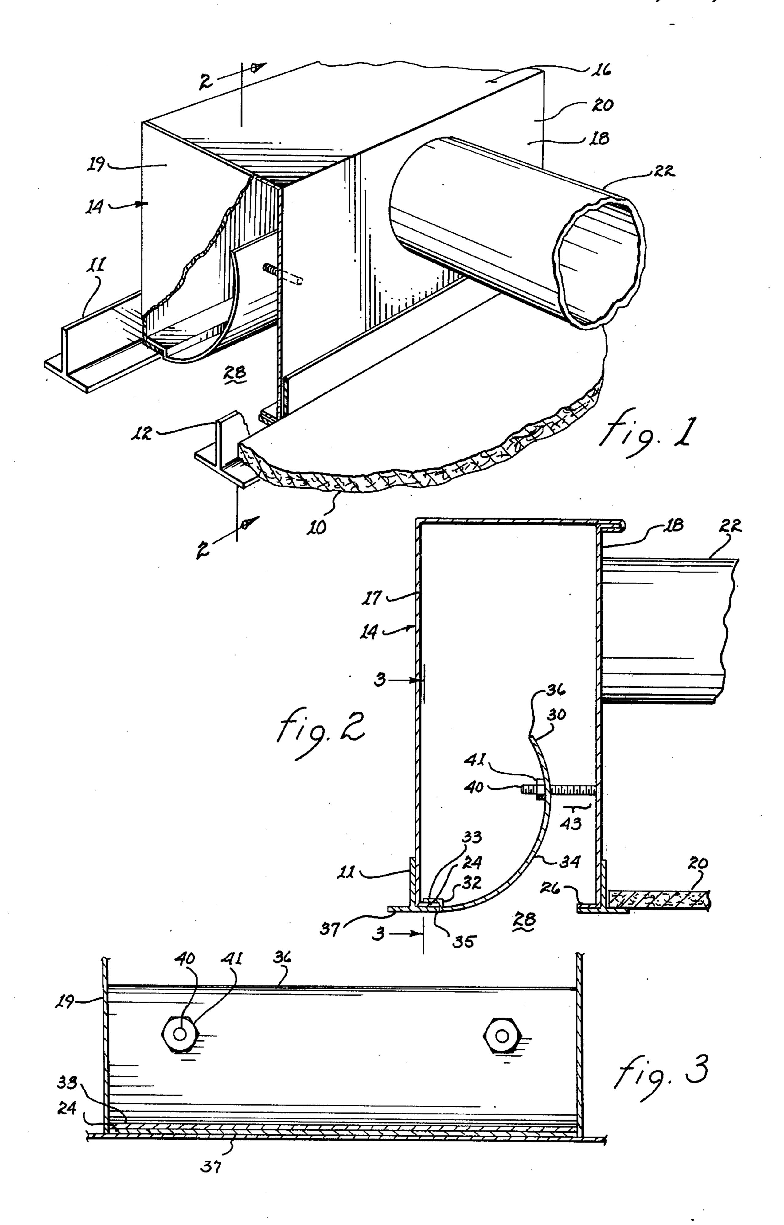
The present invention pertains to diffusers and more particularly to diffusers known as slot diffusers for use 5 in distributing conditioned air.
