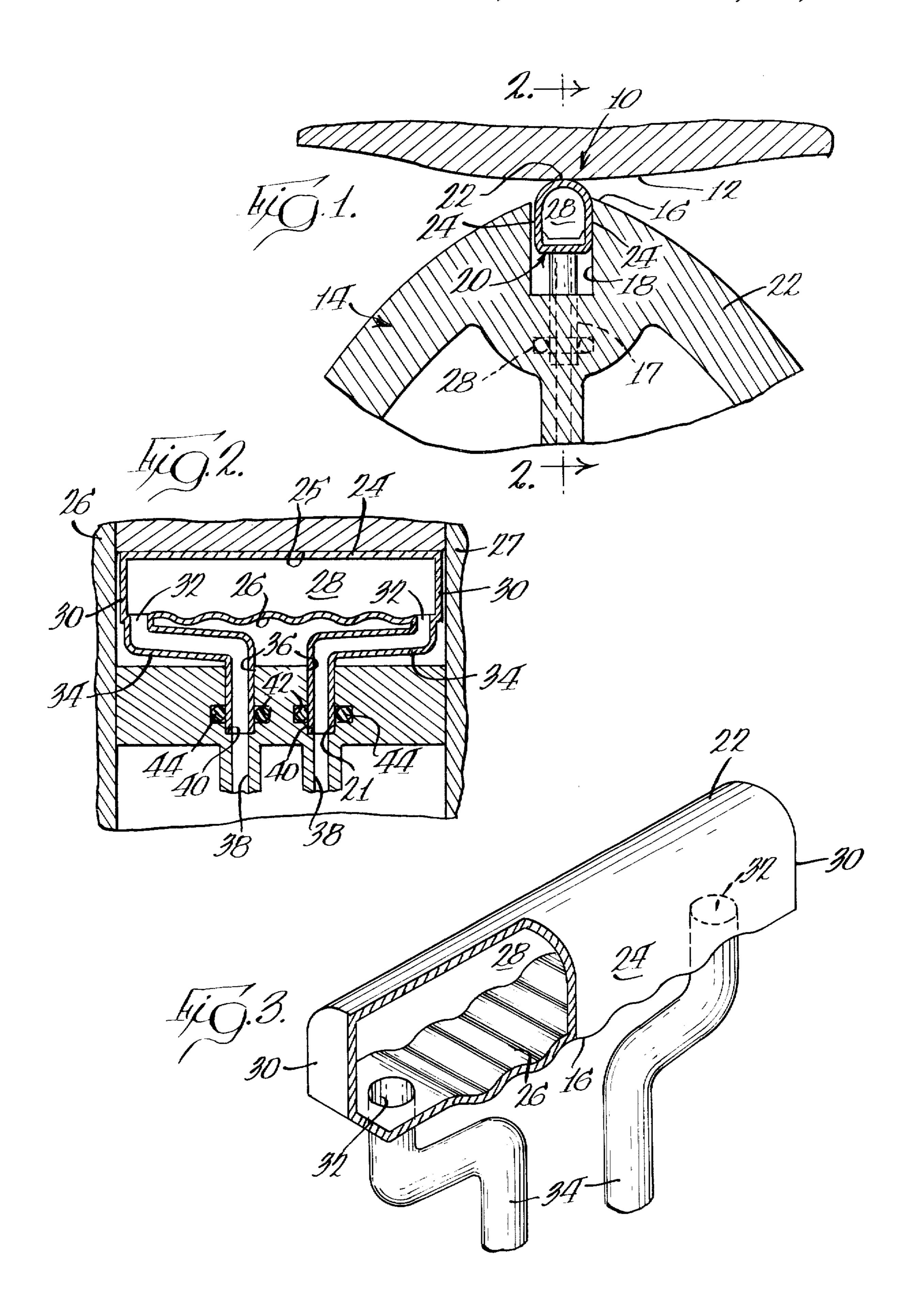
OIL COOLED SEAL FOR ROTARY ENGINE
