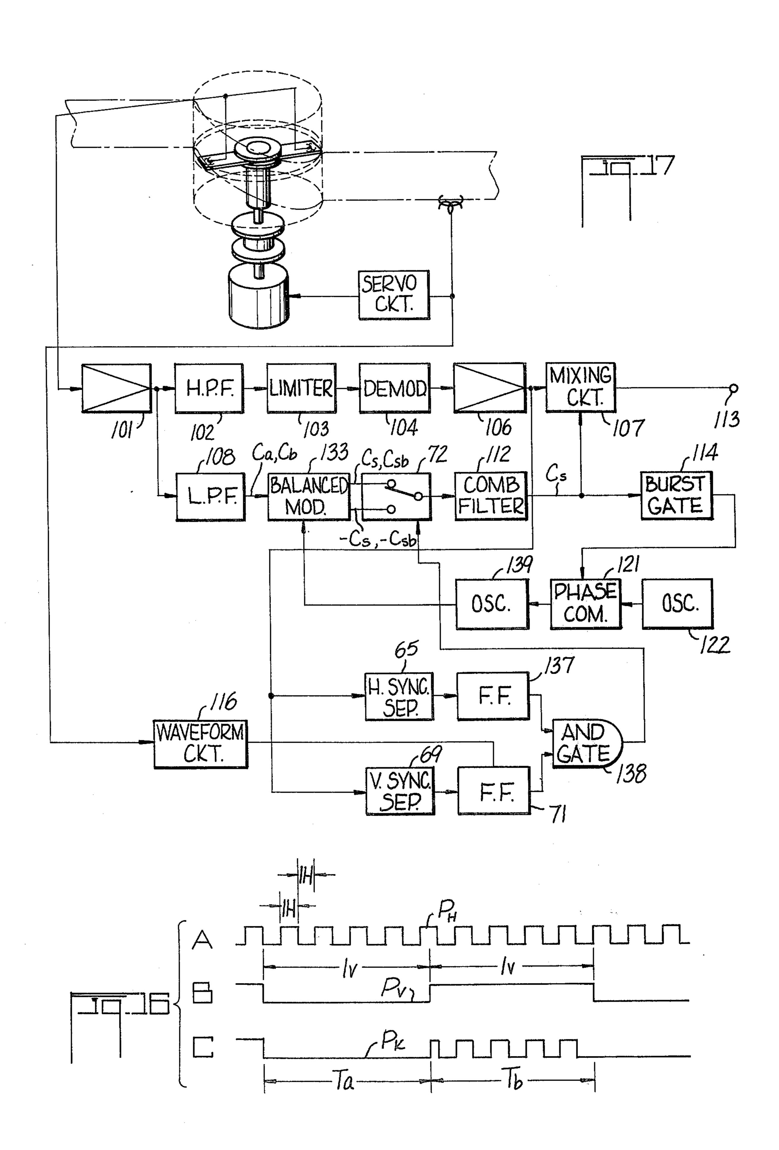
MAGNETIC RECORDING AND/OR REPRODUCING APPARATUS
