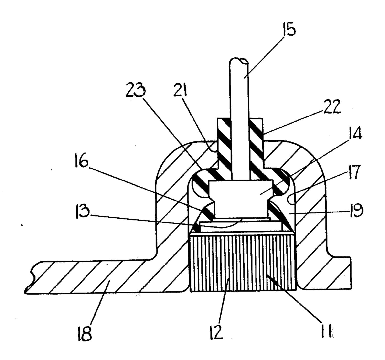
ASSEMBLY OF A RECESSED HEAT SINK AND A SEMICONDUCTOR DEVICE SEALED WITHIN THE RECESS IN THE HEAT SINK AND THERMALLY CONNECTED TO THE HEAT SINK
