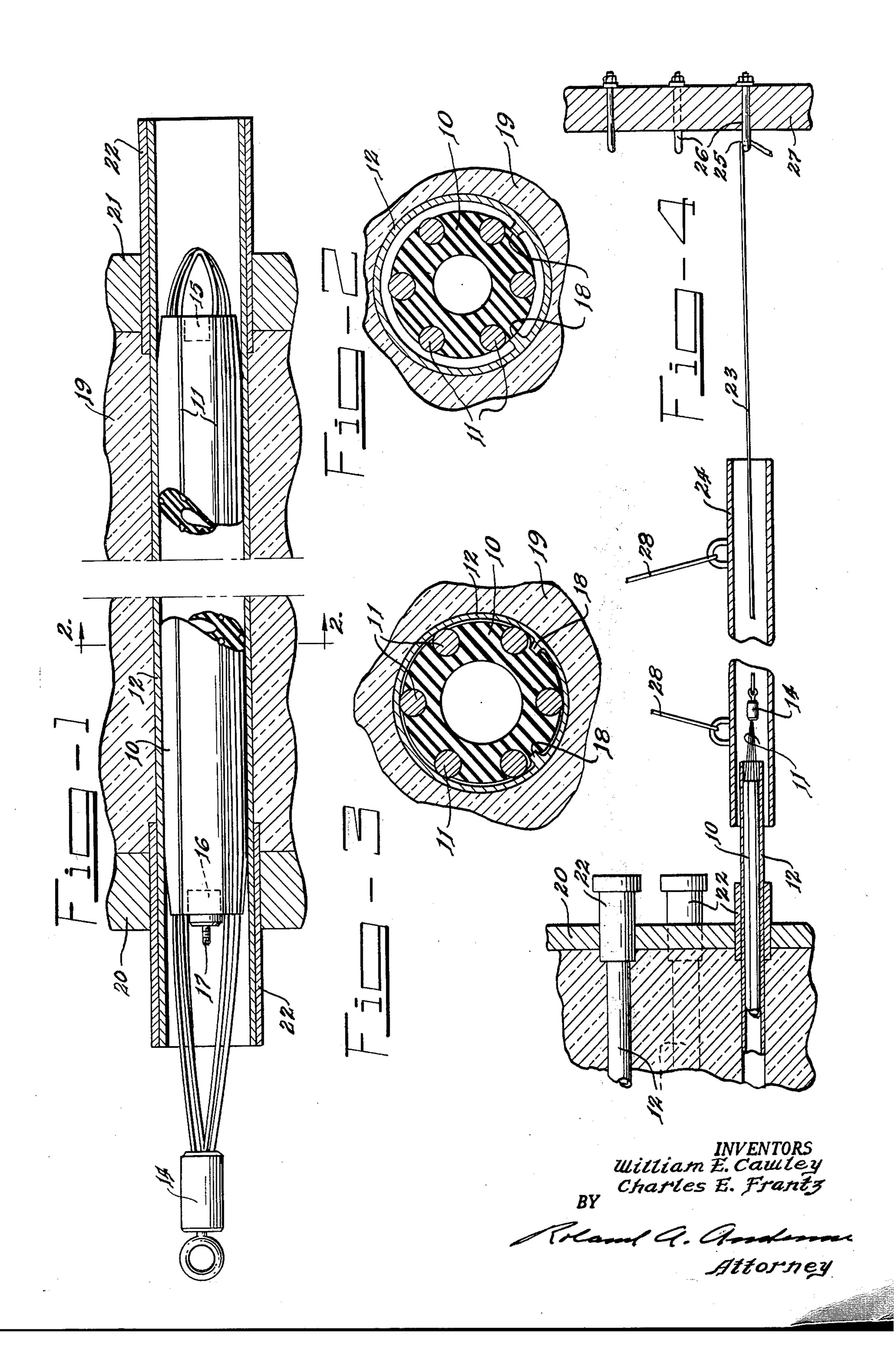
so as to protrude slightly therefrom, extending longitudinally of the rubber tube throughout the length thereof, and being equally spaced from one another about the exterior of the rubber tube so as to define substantial circumferential spaces between said cables for the full length of said tube, said cables being flexible to permit substantial flexure of said device.
