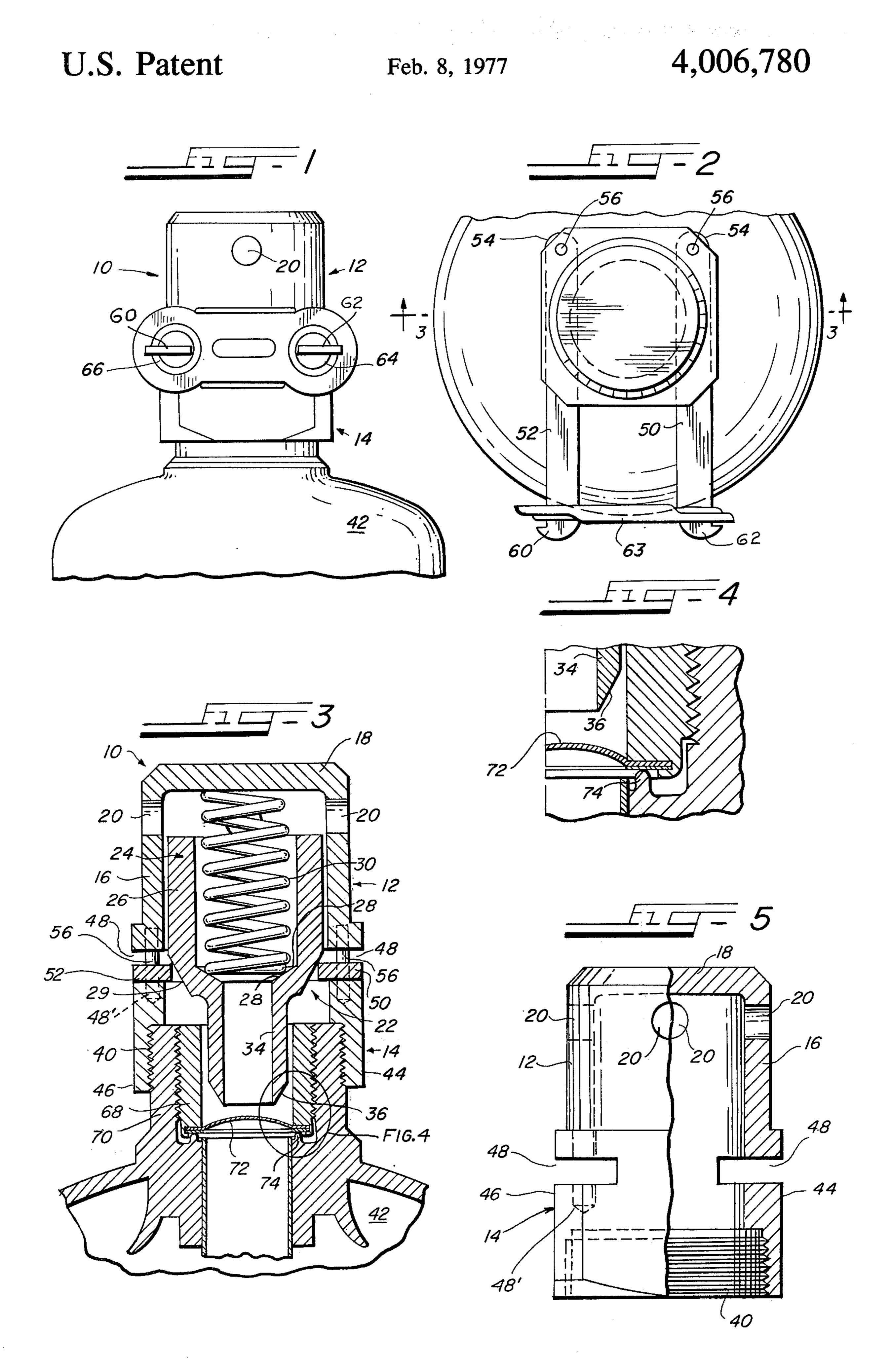
the spring bears against the lower surface of the top wall 18 of housing 10. The lower outer side wall 26 is tapered downwardly and inwardly as at 29.
