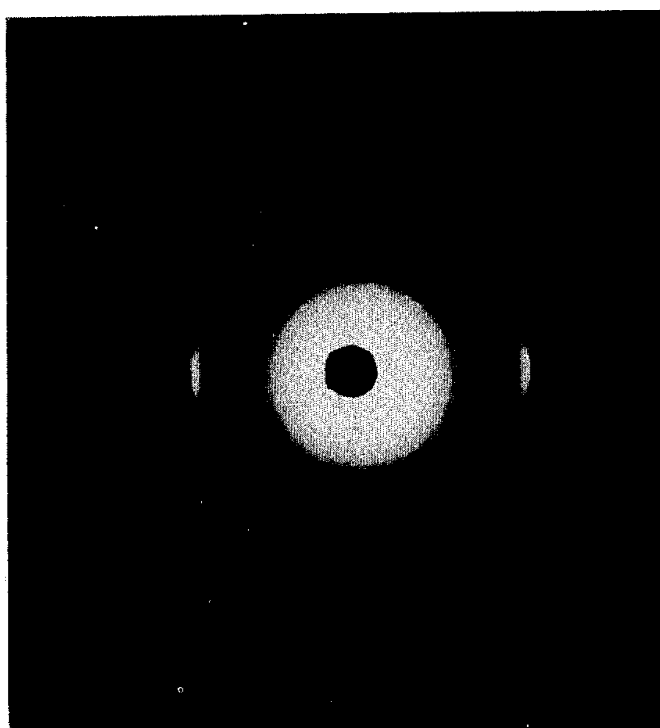
X-Ray Diffraction Pattern Petroleum Mesophase Pitch Fibers, As Drawn
