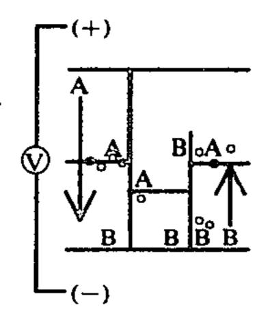
The first observed effect is that of scattering or increased opacity as the polymers A and B intermix. However, with continued application of voltage a sheet of A and a sheet of B is formed on their respective electrodes.
