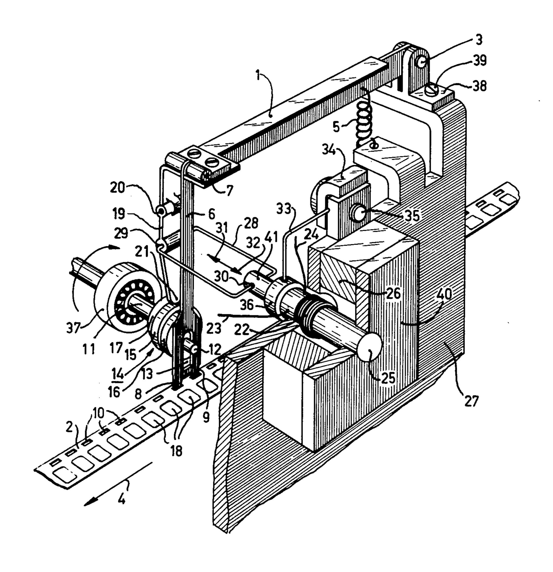
spring force and the counterfield of the electromagnet, demand the necessary adjusting operations. A further important disadvantage is moreover that with the known claw mechanism no reverse film transport is possible, unless the direction in which the drive shaft is
