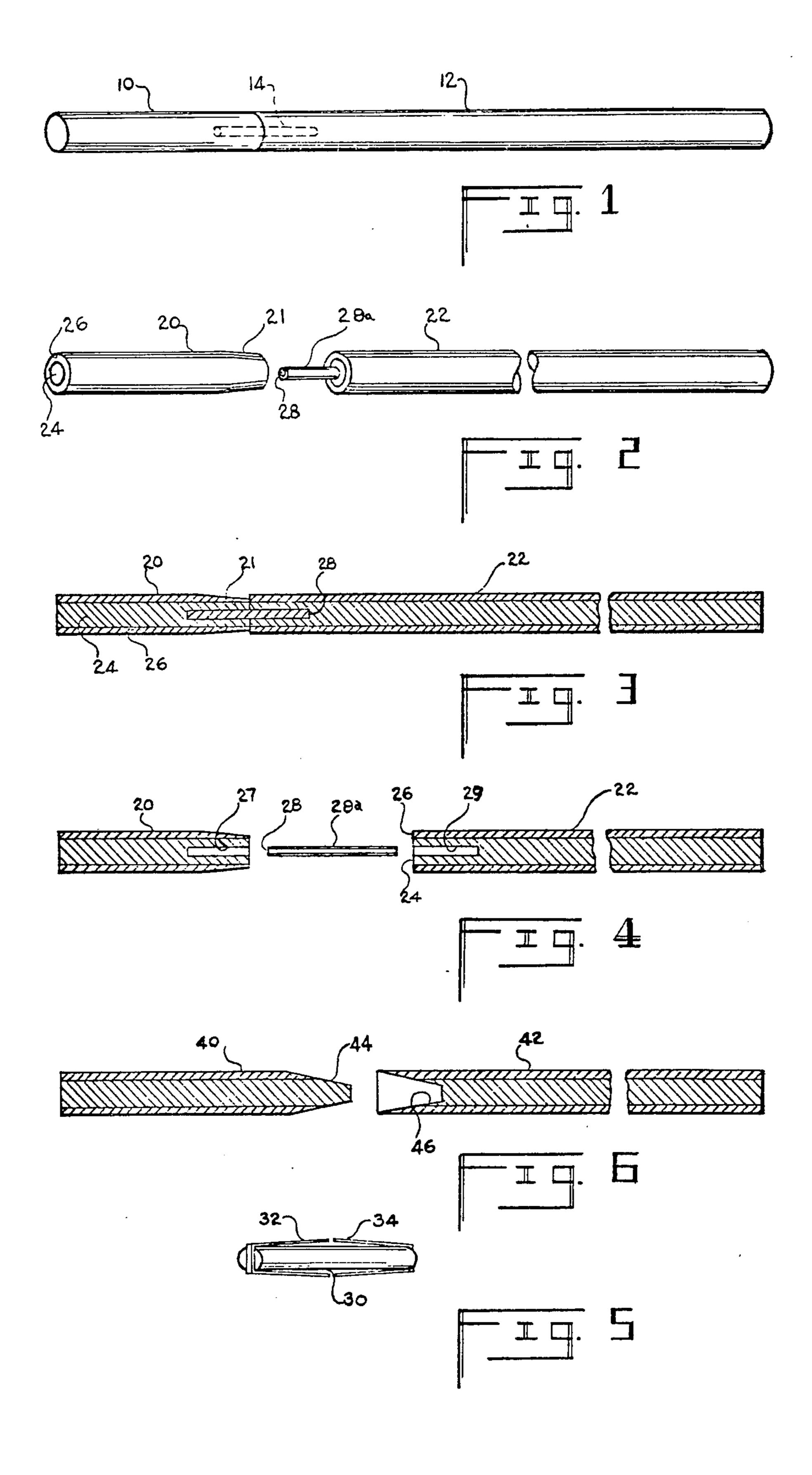
PROCESS FOR JOINING ELECTRODES AND PRODUCT RESULTING THEREFROM
