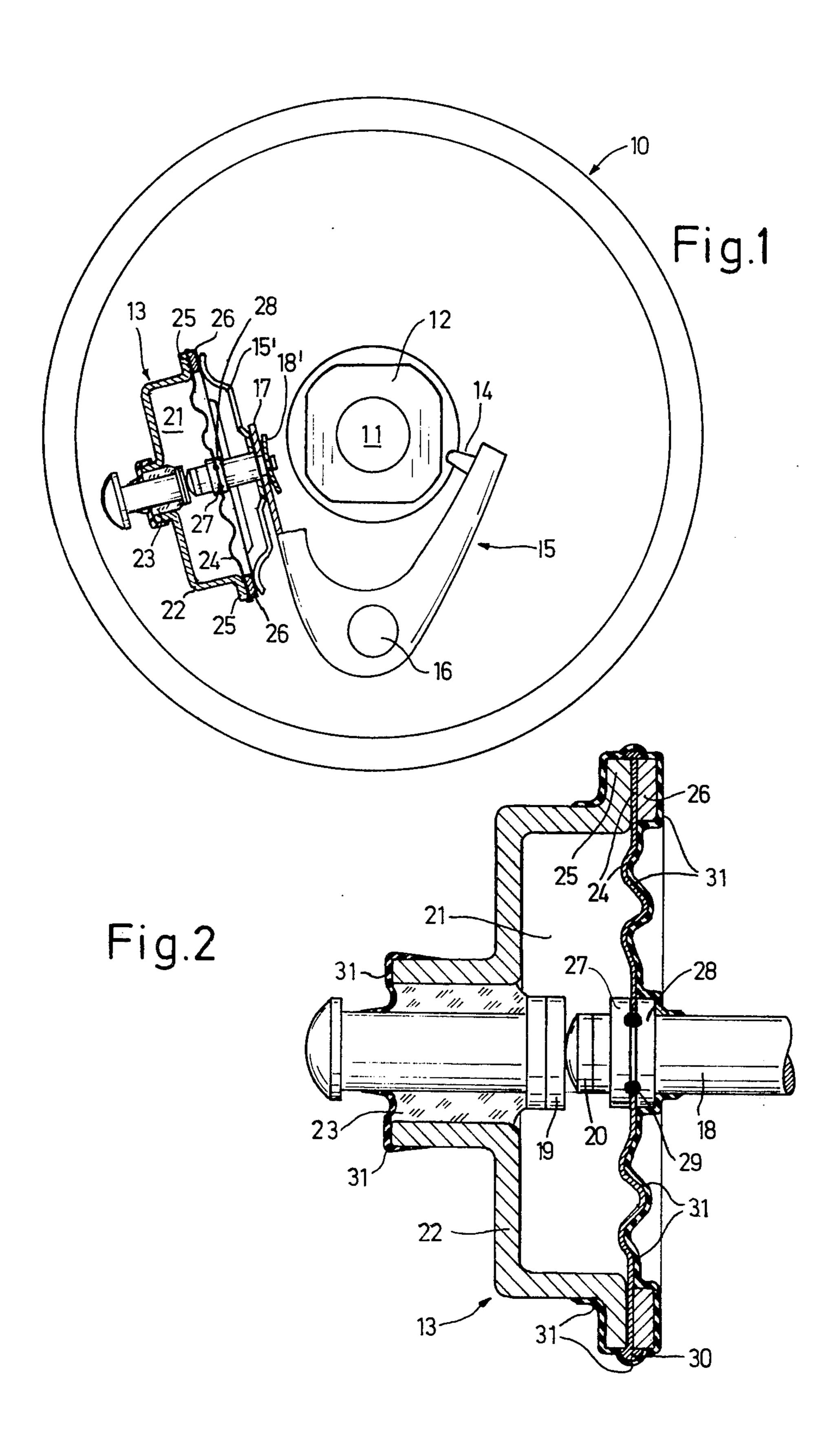
able, and the chamber 21 is gas-tight. The chamber 21, defined by the fixed housing portion 22, has a fixed contact 19 set therein, which is sealed through the
