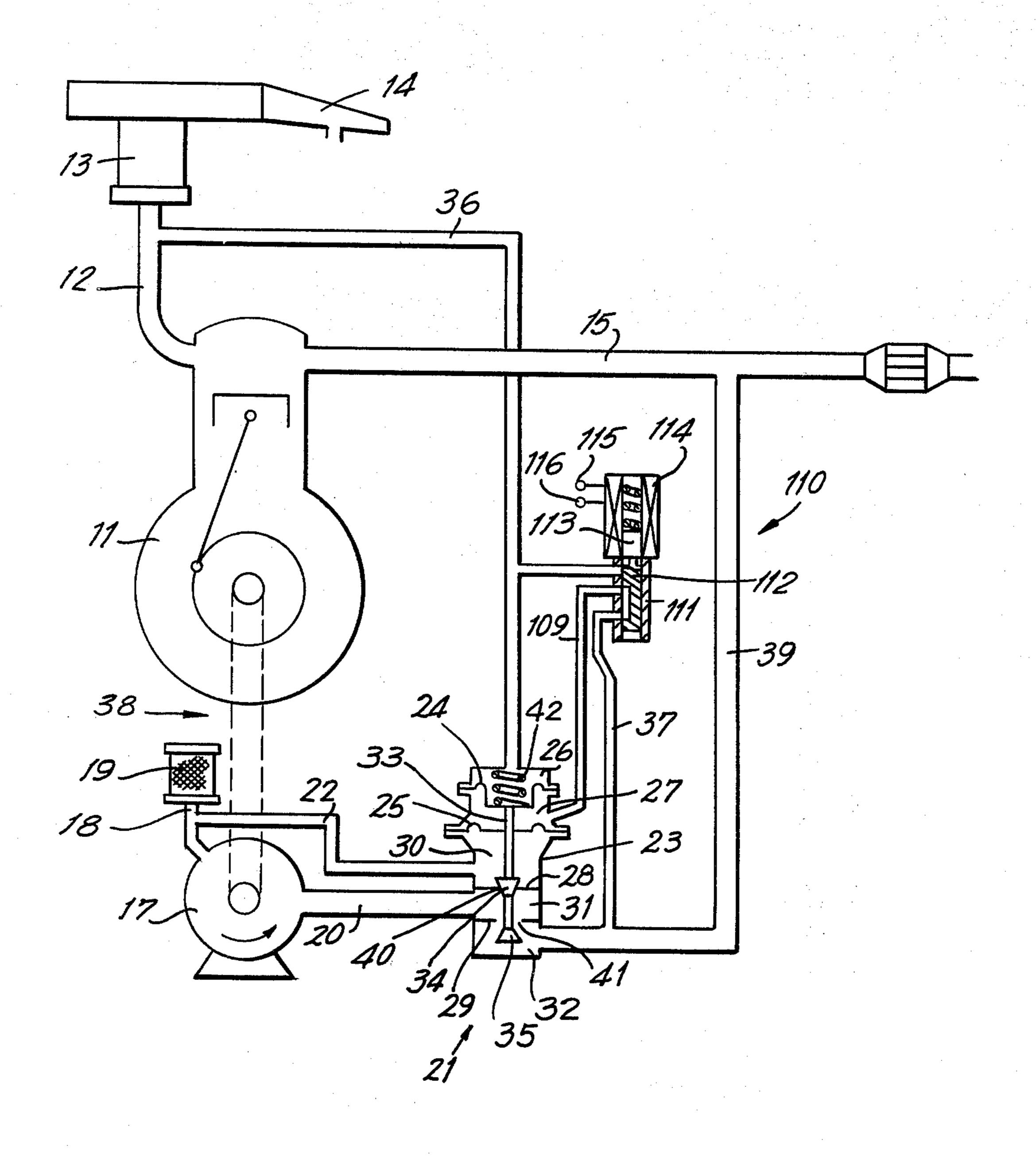
CONTROL INSTALLATION FOR THE PROPORTIONING OF A SECONDARY AIR QUANTITY FOR IMPROVEMENT OF THE COMBUSTION IN INTERNAL COMBUSTION ENGINES OR THE AFTERBURNING OF THE EXHAUST GASES OF INTERNAL COMBUSTION ENGINES
