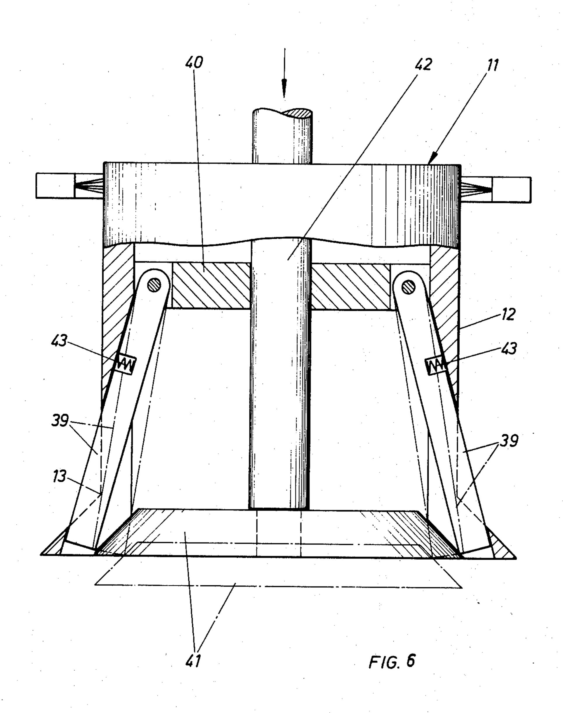
The invention relates to a delivery device for running yarn with a winding body to which the thread feeds in the range of a conical extension for the formation of a rewinding stock, the latter being displaced rearwardly and removable over head.
