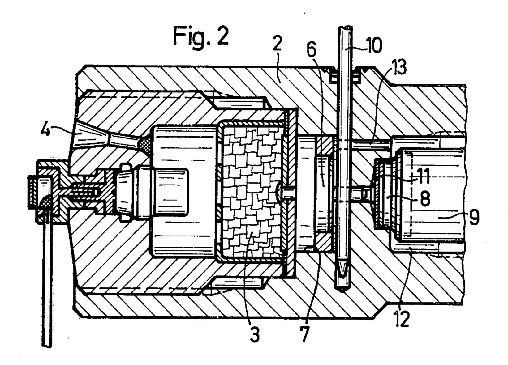
ignition of the propelling charge acts upon the disc of synthetic material to be the same on both sides so that it will not exert pressure liable to actuate the detonator cap.
