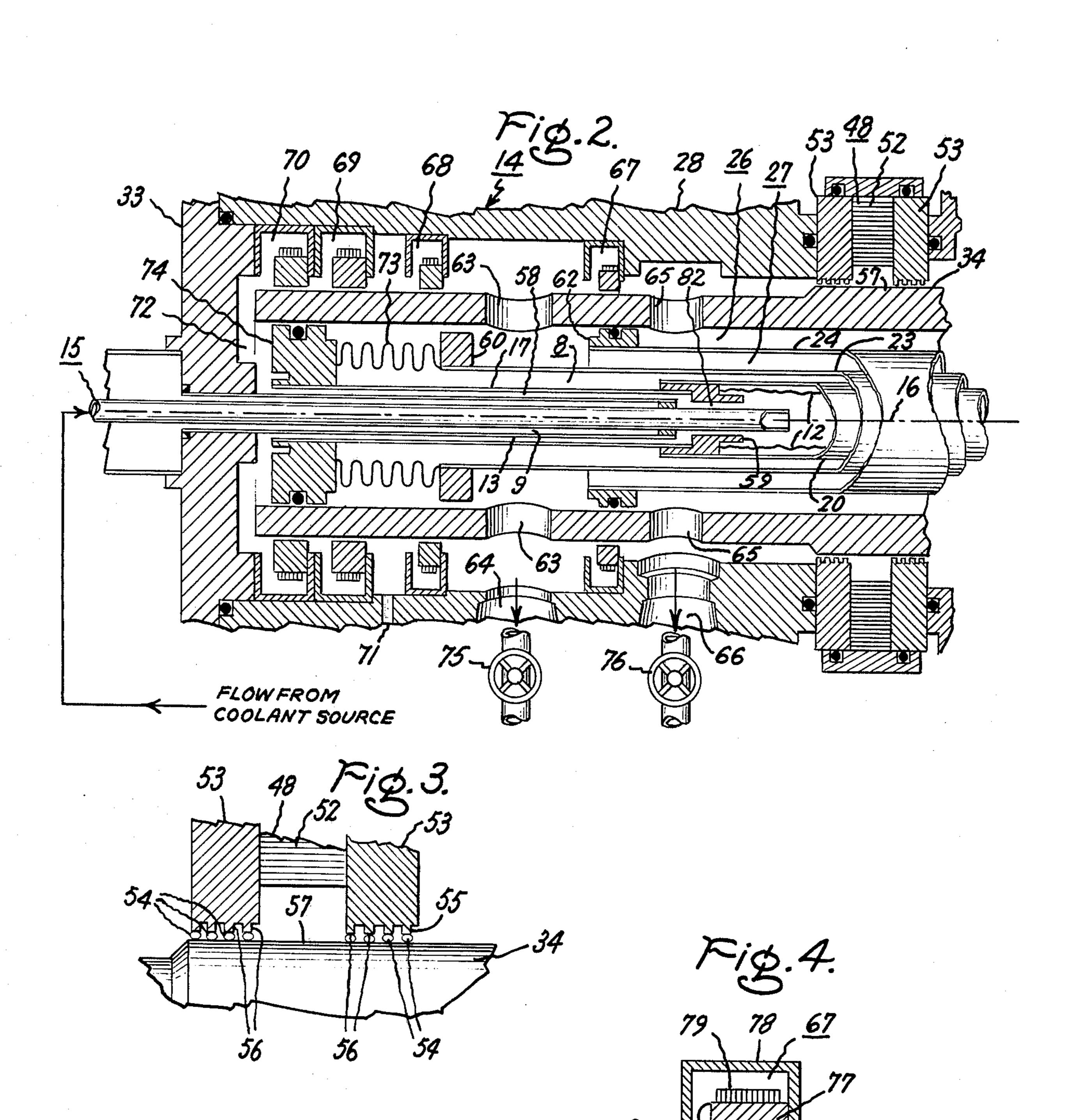
METHOD OF SUPPLYING CRYOGENIC FLUID THROUGH A TRANSFER JOINT EMPLOYING A STEPPED BAYONET RELATIVE-MOTION GAP
