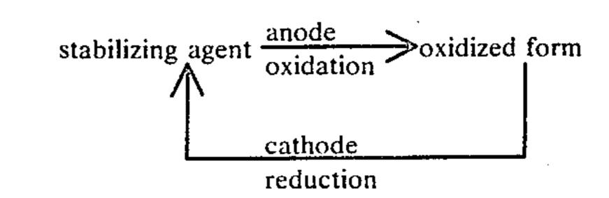
In the course of time, the only electrochemically active compound is thus the stabilizing agent itself, and this electrochemical cycle blocks and prevents any other electrochemical reaction at the electrodes, which might ineluctably lead to a degradation of the liquid crystal.
