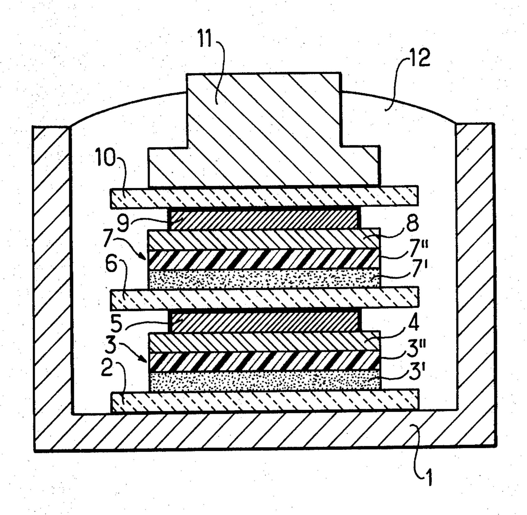
METHOD FOR PREPARING ELECTROCHEMICAL **ELEMENTS IN THIN LAYERS**
