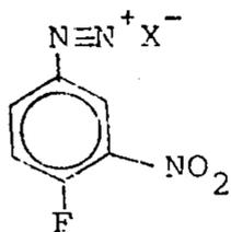
in which  $X^-$  represents a stabilizing anion are excellently suitable for the detection of urobilinogen. They represent sensitive and specific reagents for urobilinogen and do not react with bilirubin, although the sum of the Hammett sigma values of all substituents is 0.77.
