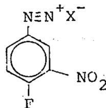
in which X<sup>-</sup> represents a stabilizing anion selected from the group consisting of a chloride, sulfate, tetrafluoroborate, hexafluoroantimonate, hexafluoroantimony sulfonate, trifluoromethyl sulfonate, aryl sulfonate, or carboxylic acid radical and at least one solid acid and optionally a wetting agent and one or several stabilizers.
