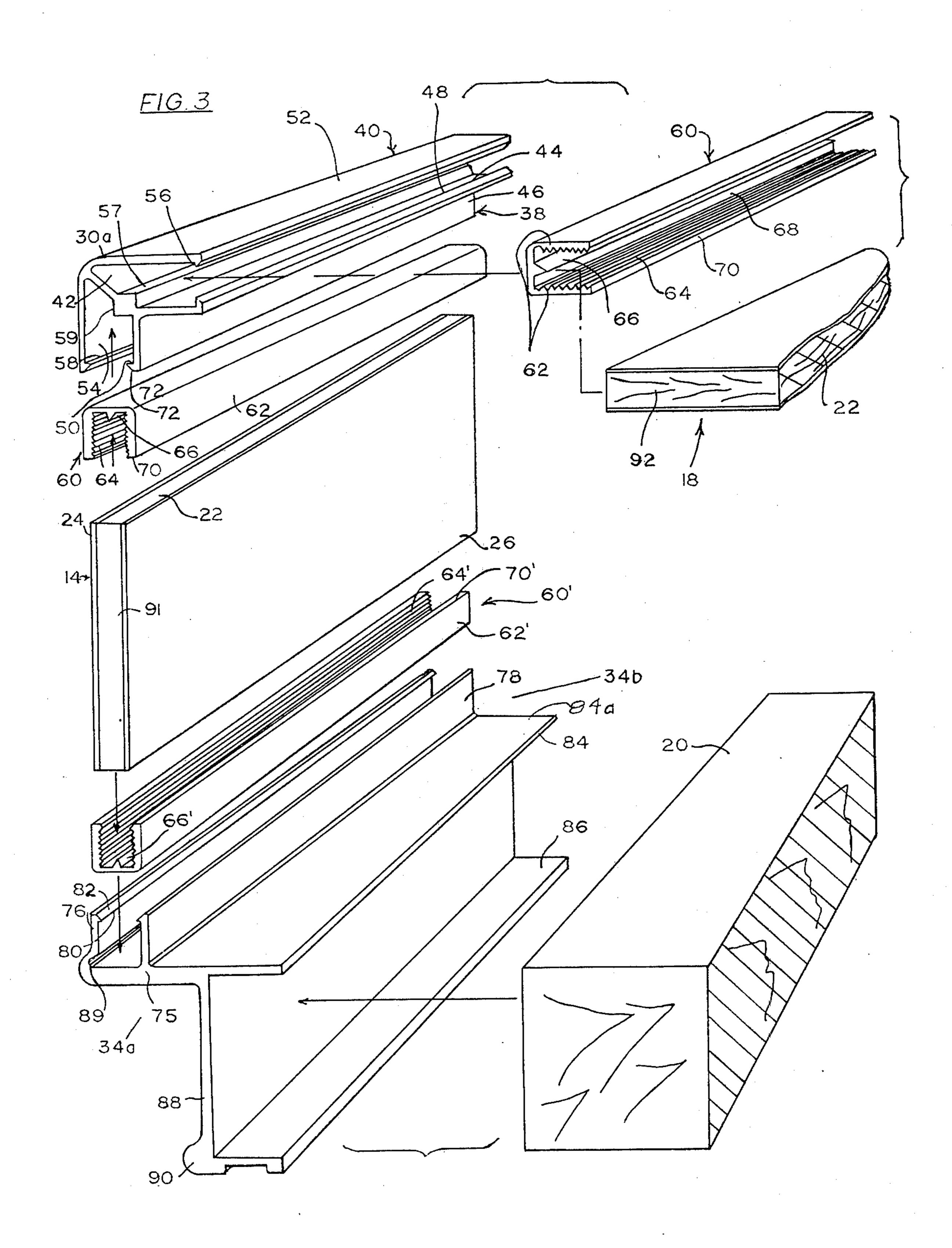
This invention relates to a panel assembly for forming a container for a transportation vehicle and more particularly concerns an assemblage of panels, moldings and rails adapted to secure the panels in mutually perpendicular planes without the use of supplementary fastening devices such as bolts or rivets.
