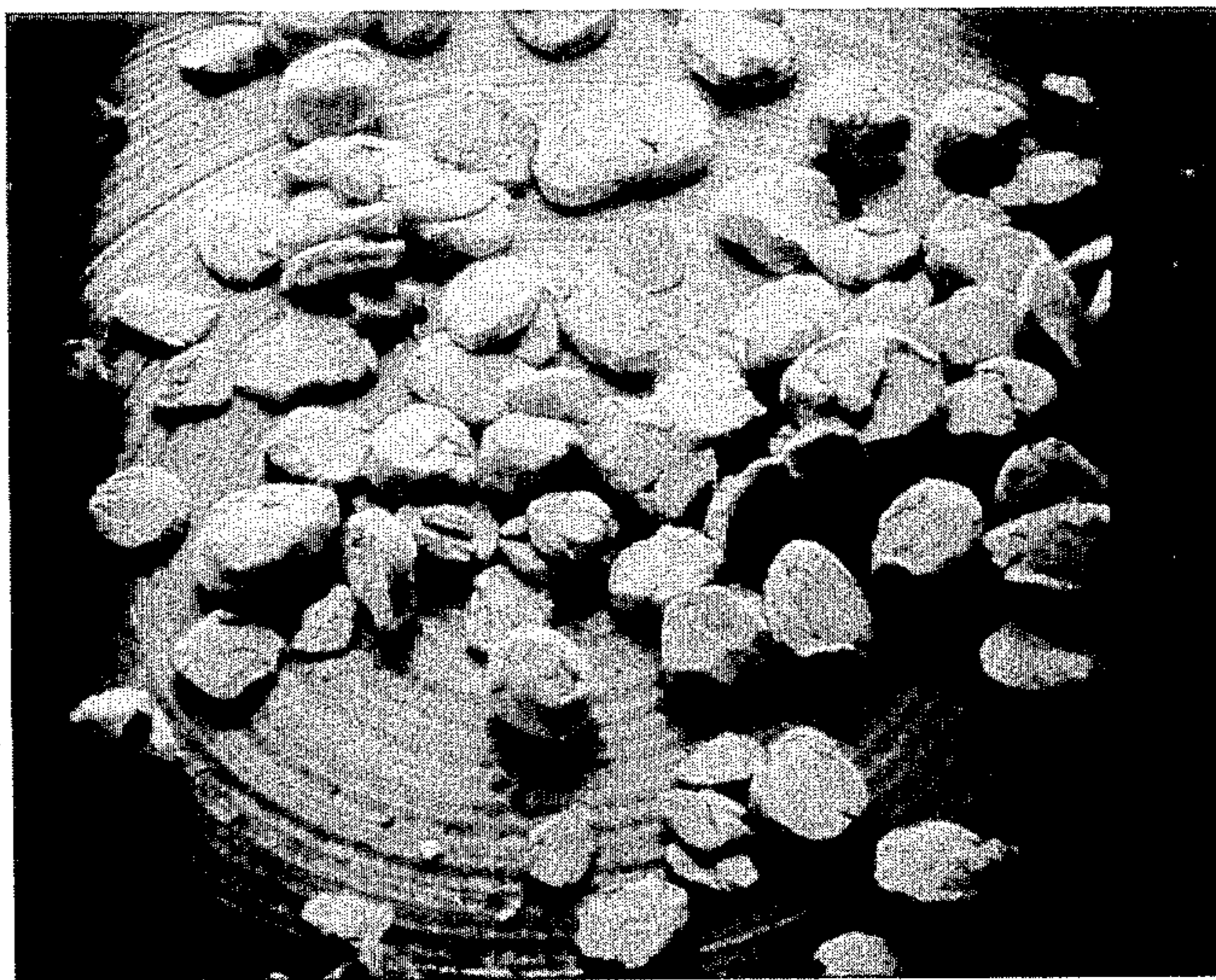
GRADE #120 ATOMIZED ALUMINUM POWDER 1mm MILLED IN BENZENE
