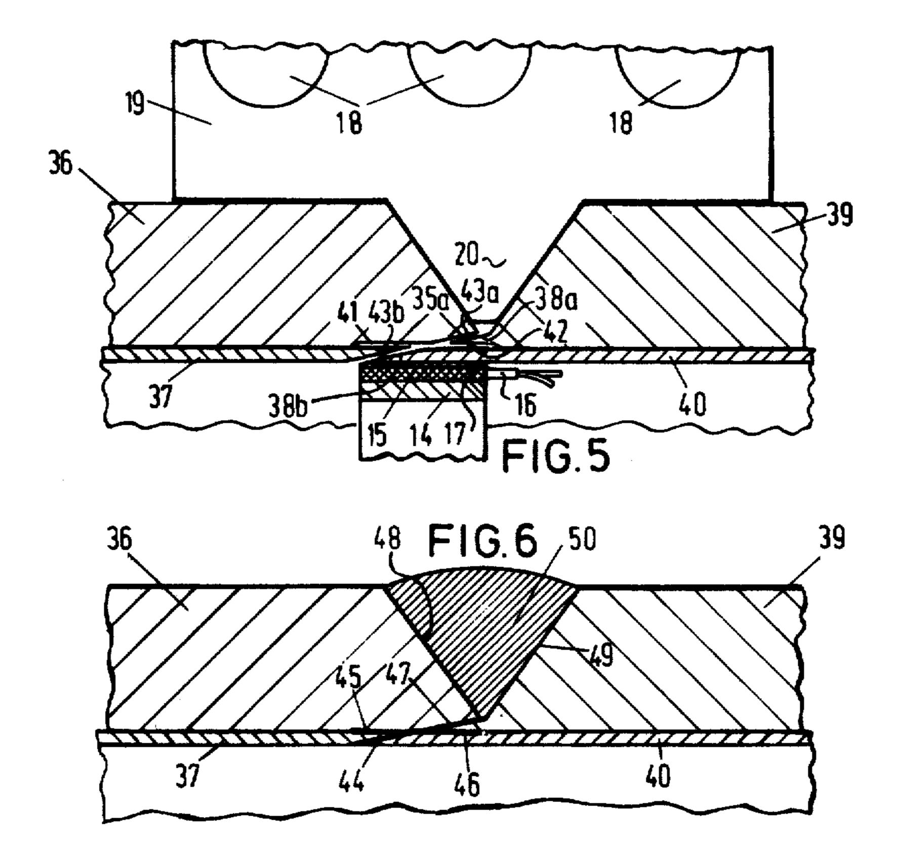
METHODS FOR WELDING TWO METAL PIECES OF TUBING WITH THEIR ENDS TO EACH OTHER AND TO PIPE-LINES CONSISTING OF PIECES OF TUBING THUS WELDED TO EACH OTHER
