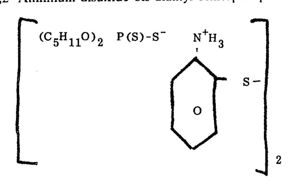
25 g (0.1 mol) bis(2-aniline) disulfide and 54 g (0.2 mol) diamyl-dithiophosphoric acid were dissolved in 100 ml toluene. The mixture was heated to 80°C. for 2 hours under nitrogen with stirring. Removal of toluene in vacuum yielded the reaction product. Elemental Analysis:
