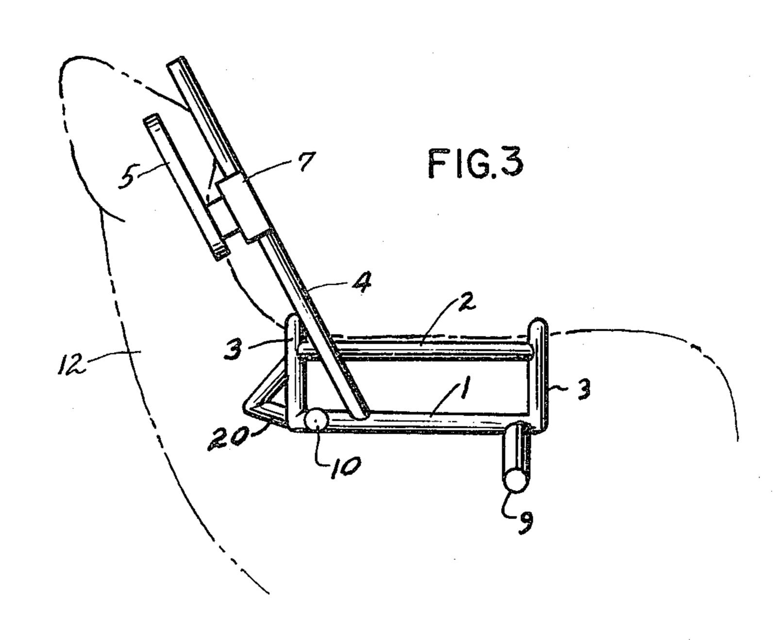
tion, there is a semicircular jaw holder attached to the end of holder bar 4, the present invention eliminates such jaw holder.
