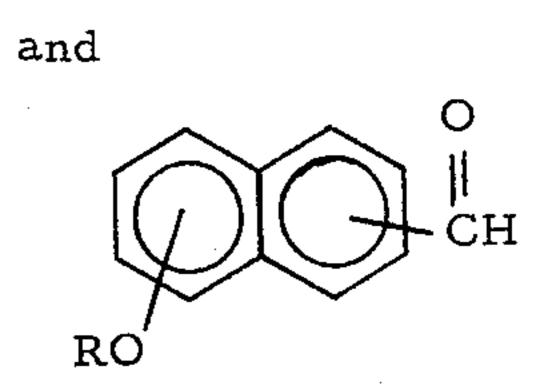
where R is methyl, ethyl, propyl, or isopropyl, and including from 1 to about 97 percent of at least one compound selected from the group consisting of alpha unsaturated carboxylic acids, amides, and esters for 5 producing bright electrodeposits of tin from an aqueous, acid plating bath.
