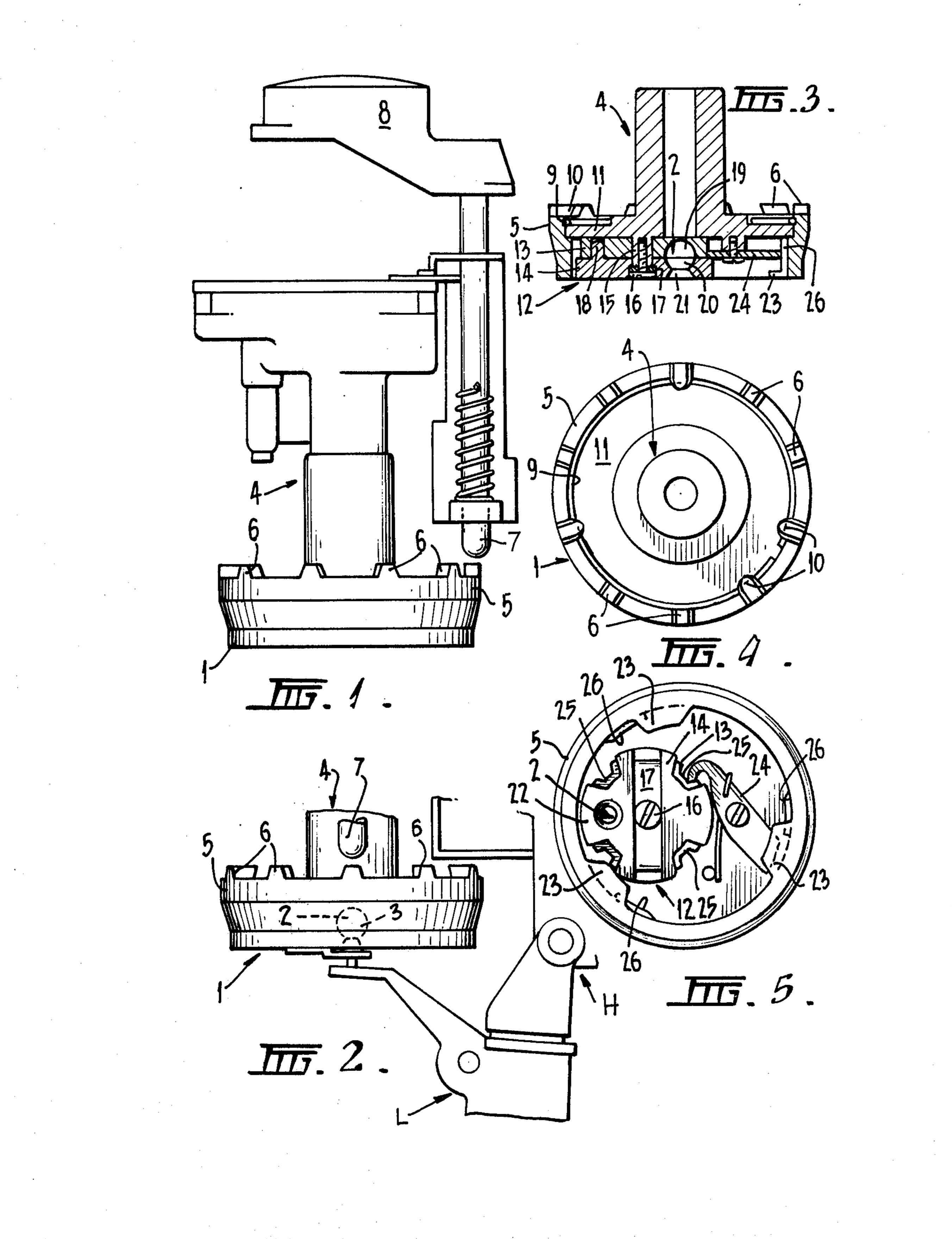
able pivot member for adjusting the degree of oscillation of the head.
