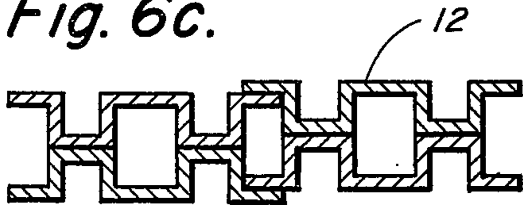
TWO-LAYER ROOF OR WALL
