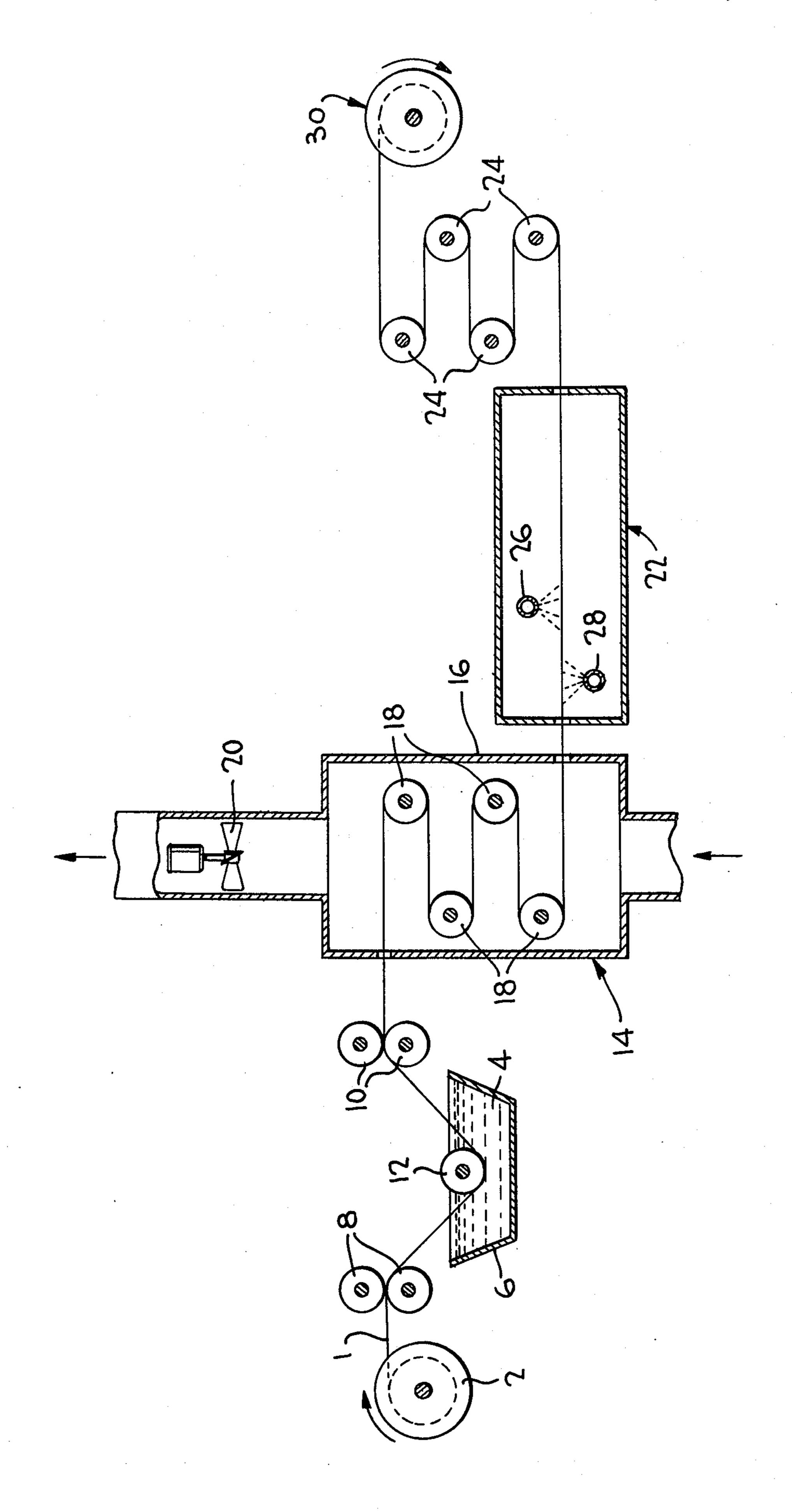
PROCESS FOR DRAWING ACRYLIC FIBROUS MATERIALS TO FORM A PRODUCT WHICH PARTICULARLY IS SUITED FOR THERMAL STABILIZATION AND CARBONIZATION
