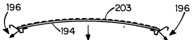
FINISHED WORKING SCREENING MASTER WITH GRILLE OR PHOSPHOR MASTER STENCIL PATTERN
