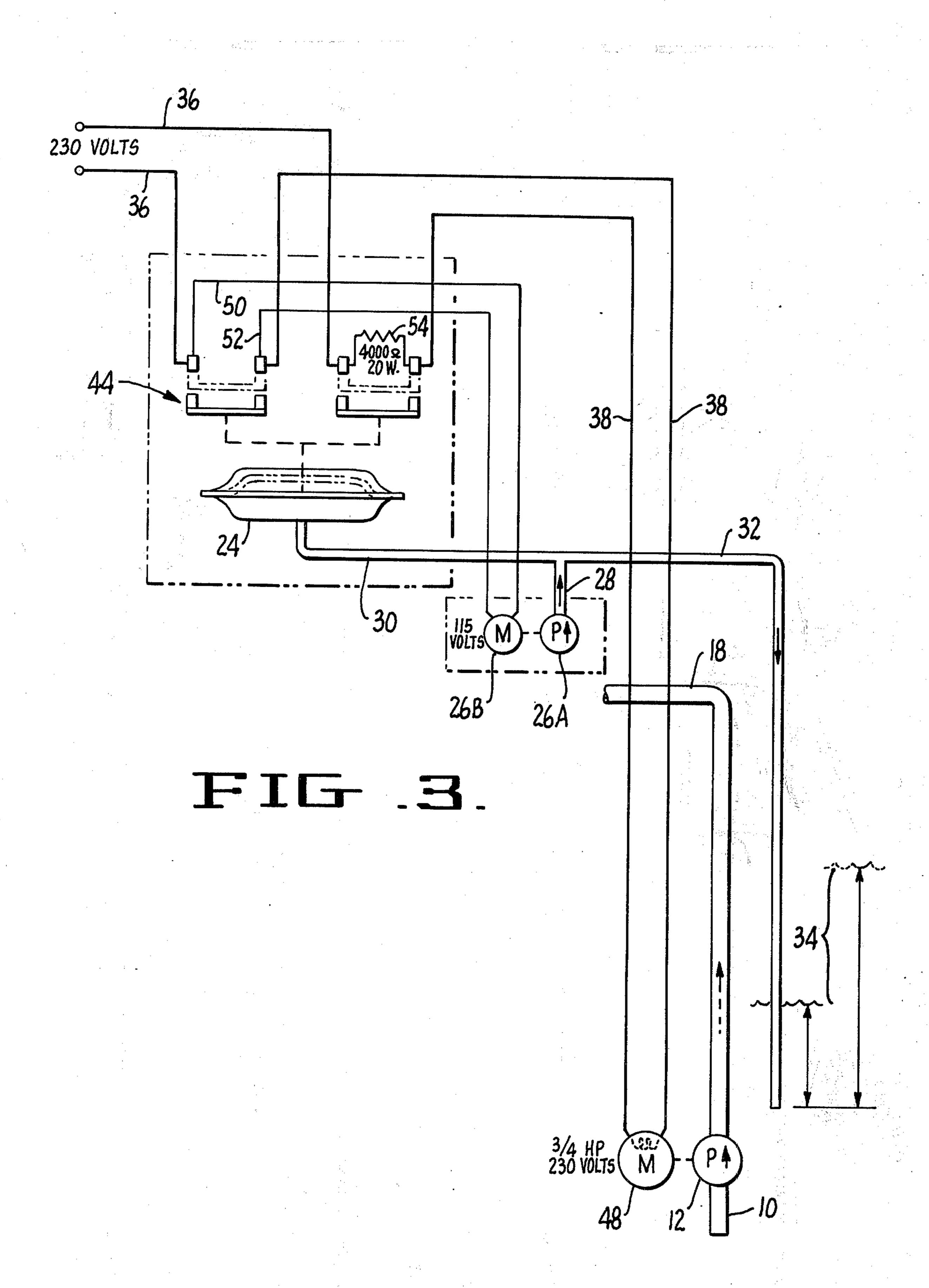
Among the objects and advantages of the invention are the following: to provide protection against pump damage; to prevent the loss of pump prime; to maintain fairly precise control over liquid levels; and to locate within one compact, above-ground assembly all of the control elements except an air pressure tube which extends into the well.
