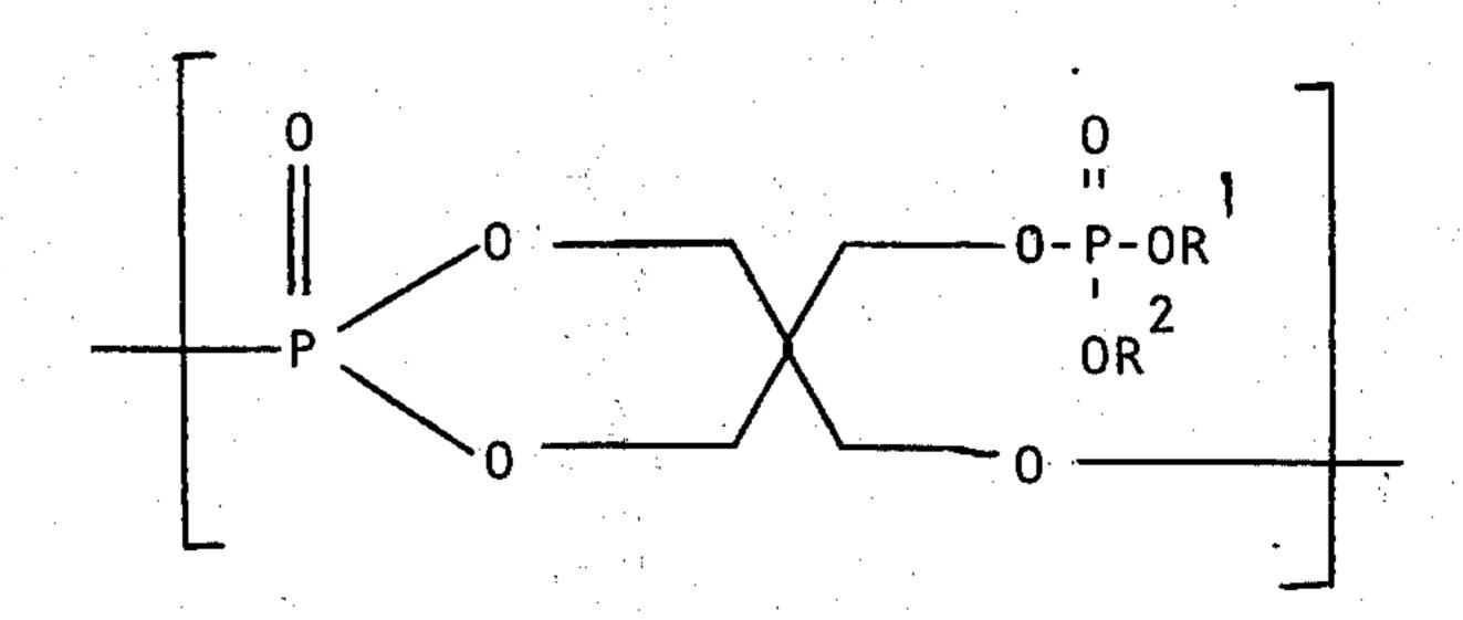
wherein the R groups are alkyl radicals, m and n are each integers from 0 to 4 and the sum of m + n is from 1 to about 4, are useful as flame retardants, especially for rigid polyurethane foams.
