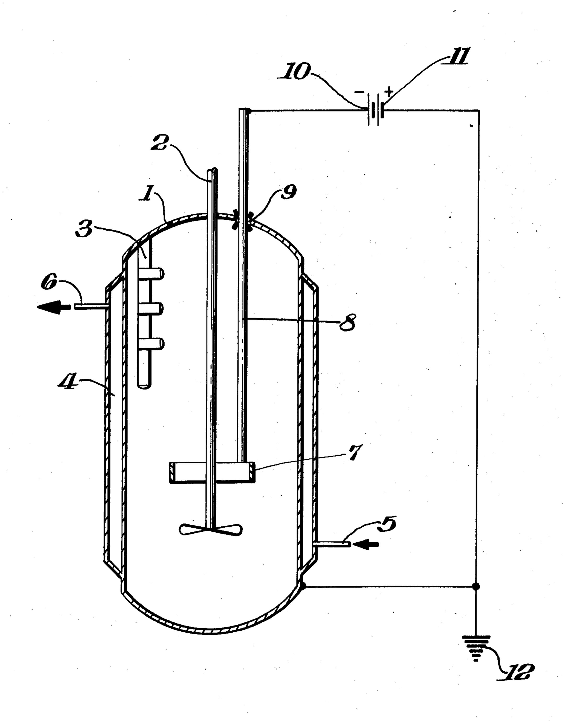
The present invention relates to an improvement in the process for polymerizing vinyl chloride in suspension in reactors lined with stainless steel or a noble metal to reduce the formation of wall deposits; it also relates to a reactor suitable for carrying out the said process.
