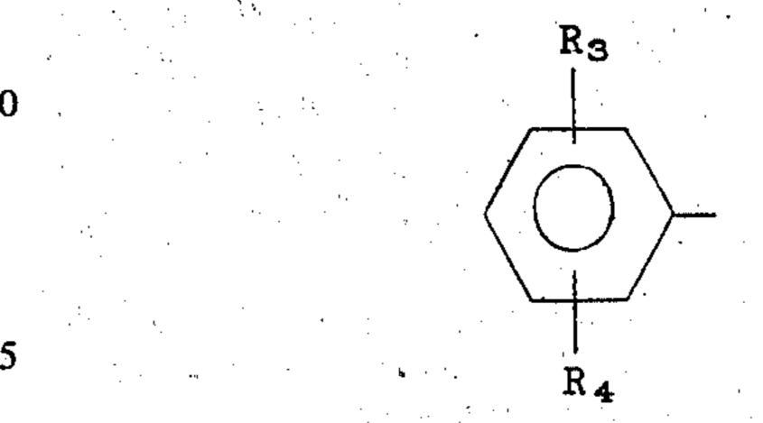
wherein  $R_3$  and  $R_4$  are monovalent groups independently selected from the group consisting of hydrogen, halo,  $C_1$ – $C_3$  alkyl, and  $C_1$ – $C_3$  alkoxy.
