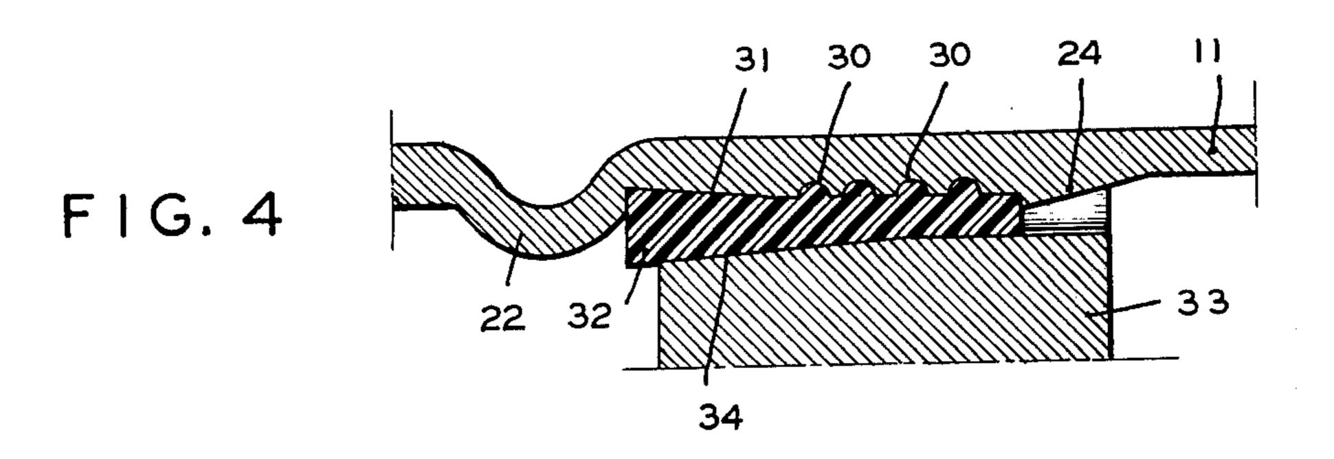
This invention relates to tire valve cores and more particularly to such cores which include a barrel which is surrounded, intermediate the extremities thereof, by resilient sealing means in the form of a plastic gasket.
