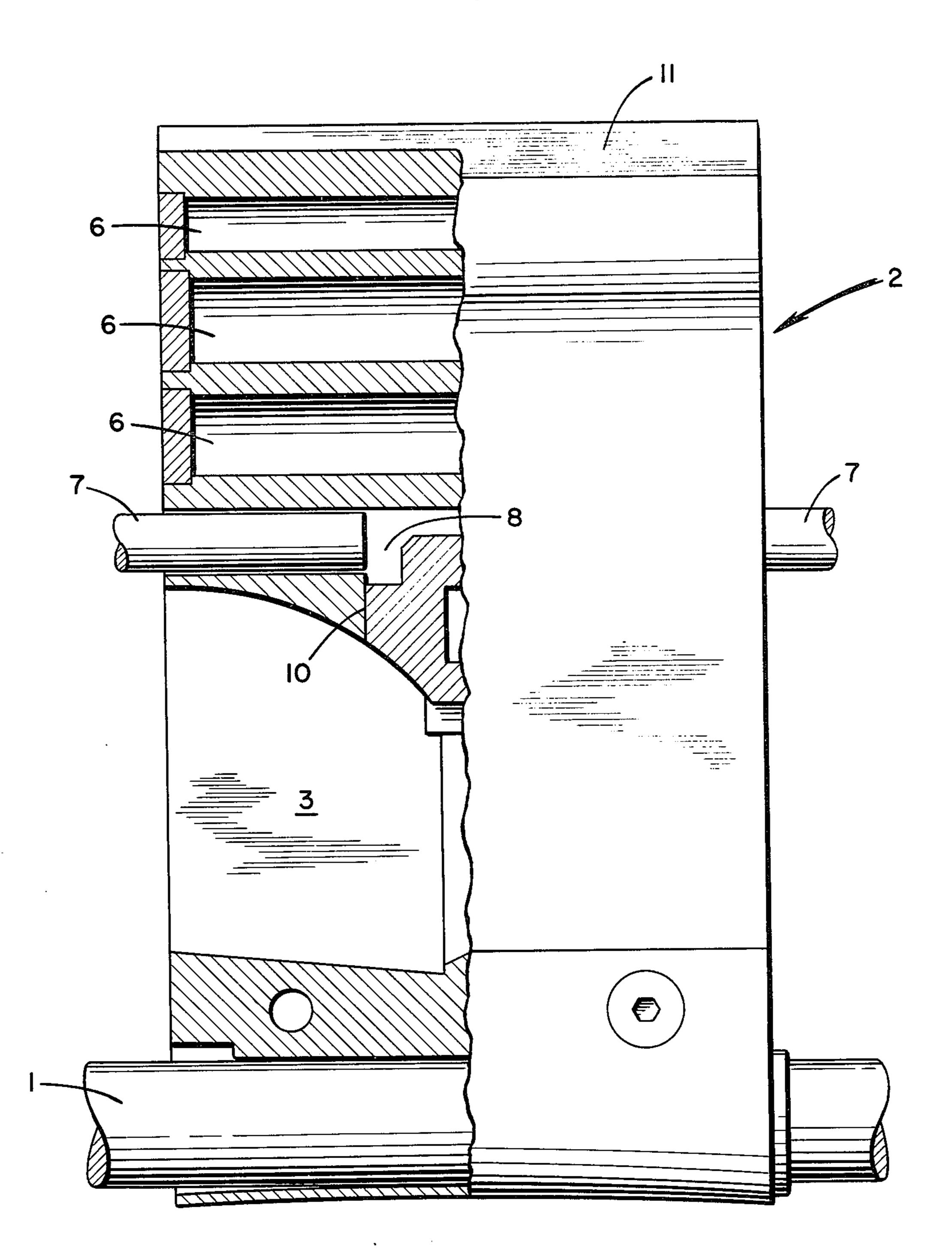
FAIRINGS FOR CABLES FOR THE TOWING OF AN IMMERSED BODY
