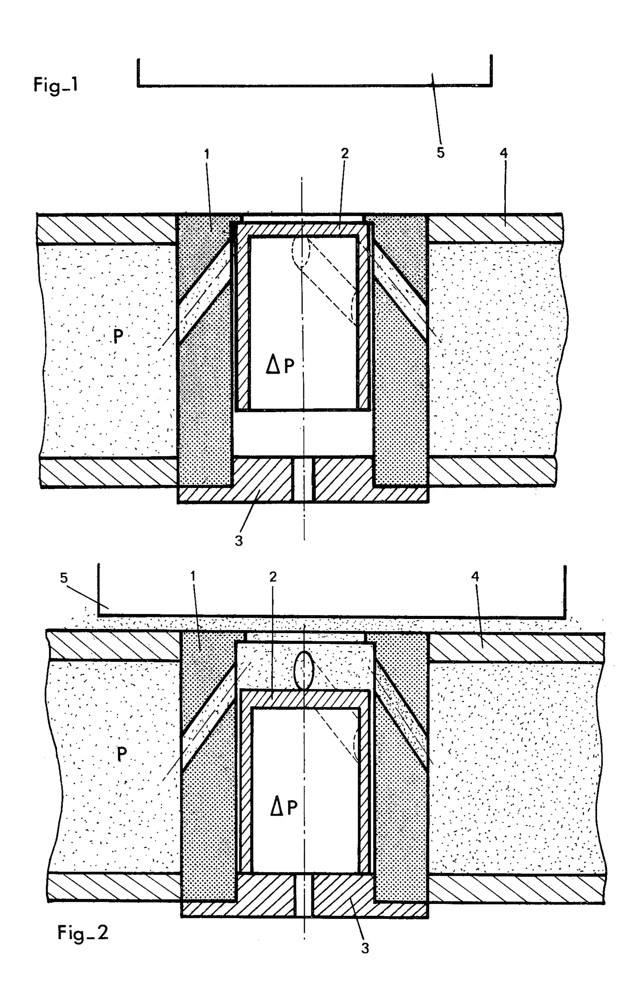
The present invention relates to air-cushion conveyors the air-cushion of which causes, under any load, opening of valves thus ensuring renewal of the air-cushion.
