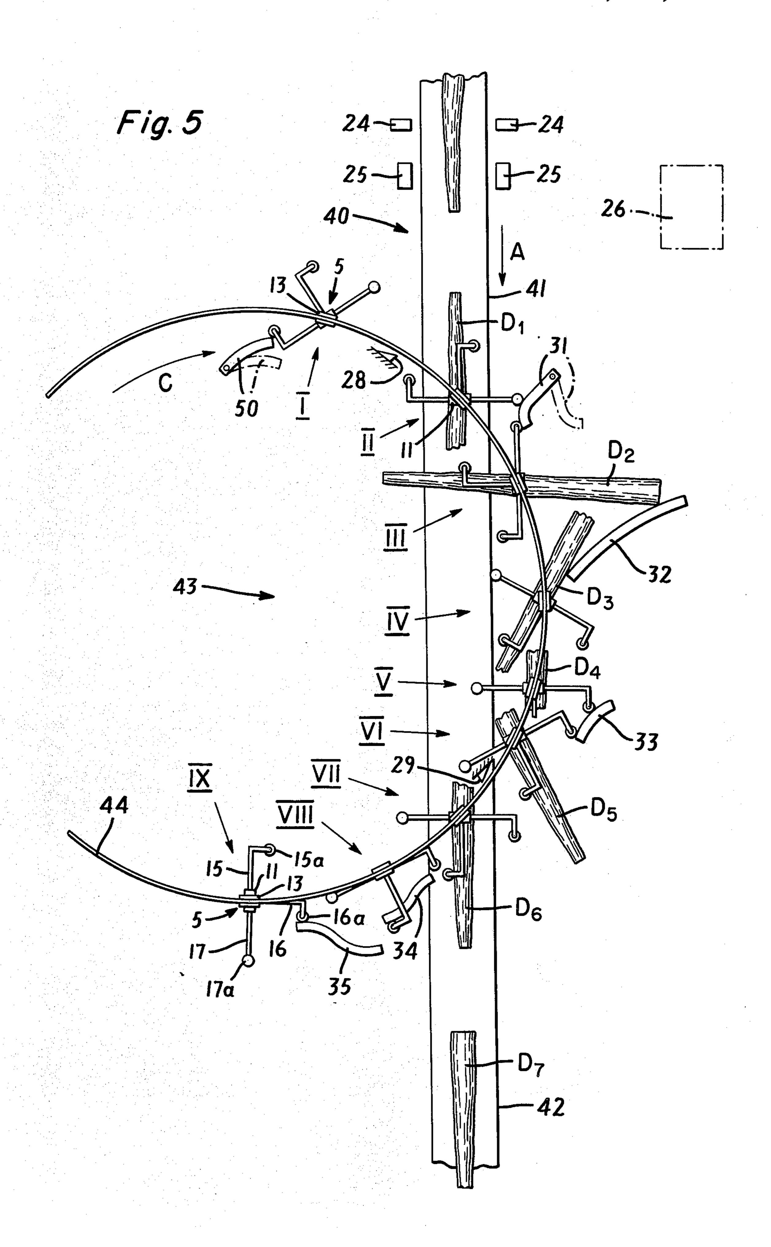
METHOD AND APPARATUS FOR TURNING LOGS
