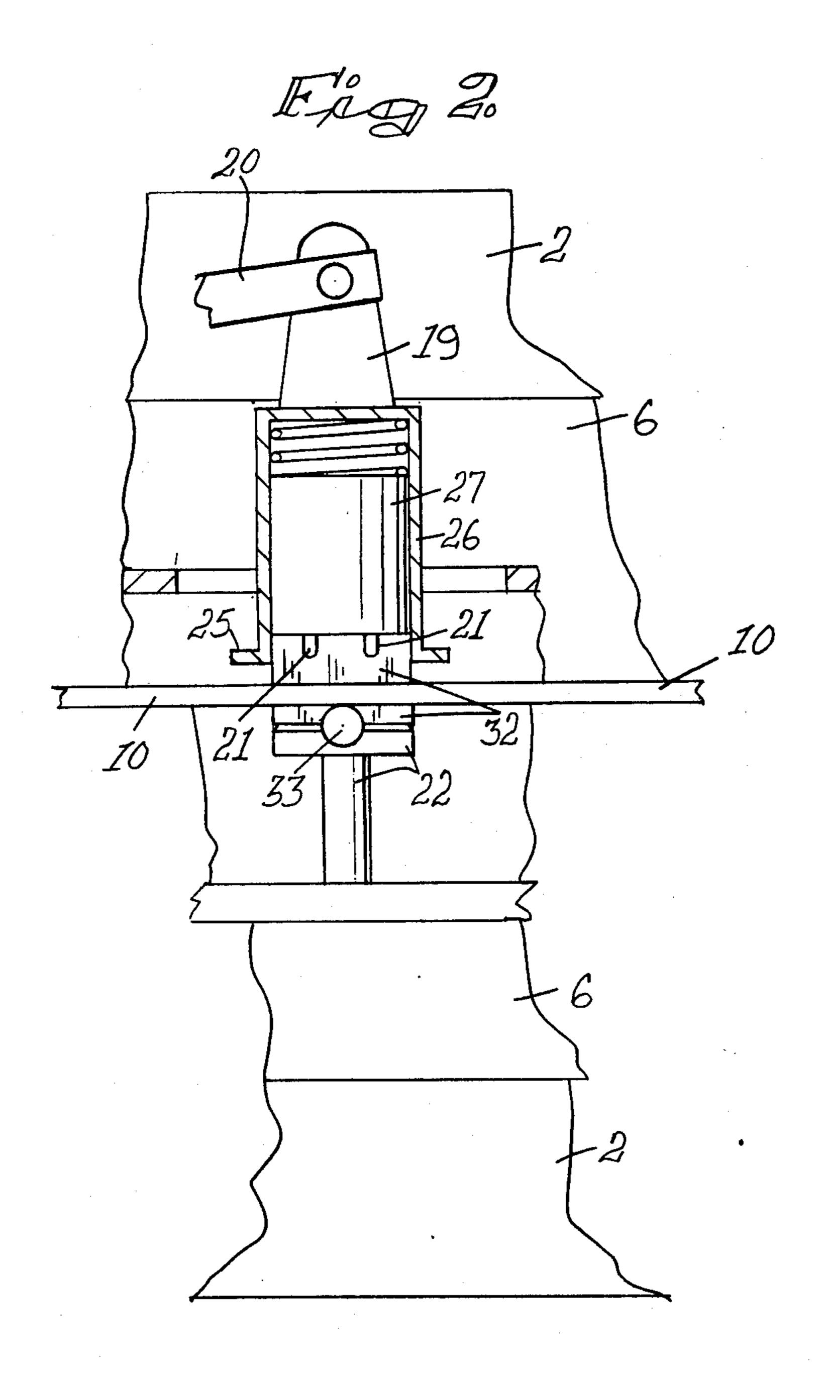
This invention relates to metal punching machines and more particularly to machines adapted to punch a series of generally equally spaced holes along the length of a piece of metal, especially metal in strip form.
