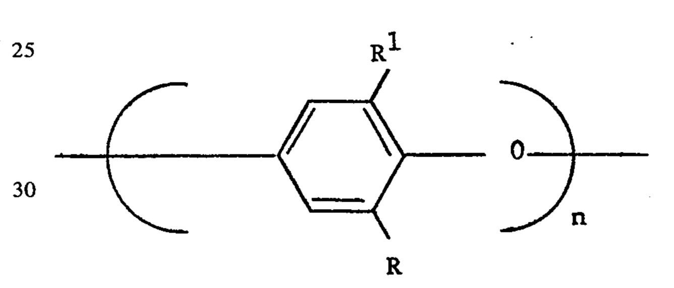
wherein R and R<sup>1</sup> are monovalent substituents selected from the group consisting of hydrogen, halogen, hydrocarbon radicals, halohydrocarbon radicals having at least two carbon atoms between the halogen atom and the phenyl nucleus, hydrocarbonoxy radicals and halohydrocarbonoxy radicals having at least two carbon atoms between the halogen atom and the phenyl nucleus, said radicals being free of a tertiary alpha-carbon atom, and n is a whole integer of at least 50.
